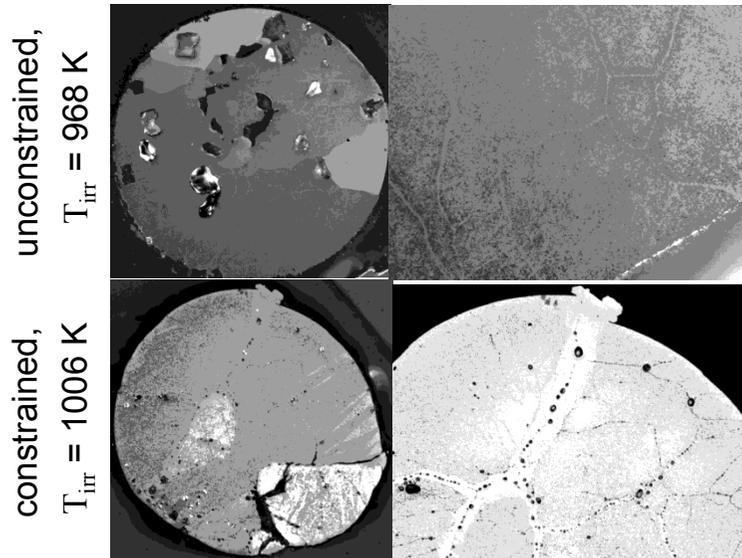
Unconstrained pebbles: large pores ( $\sim 40\mu\text{m}$ )
