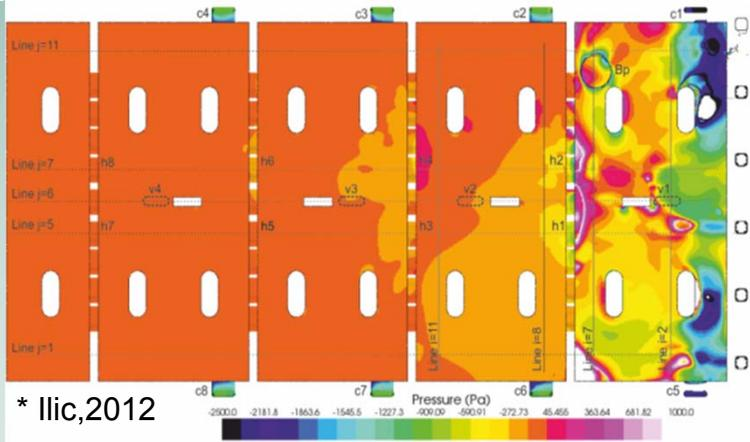
**Flow distribution of TBM manifold system simulated and verified against experiment in 1:1 fabricated mock-ups**
