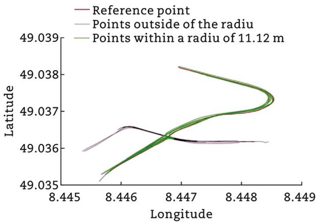
**Fig. 9 – Results of our experiment and the application of the range search algorithm.**
