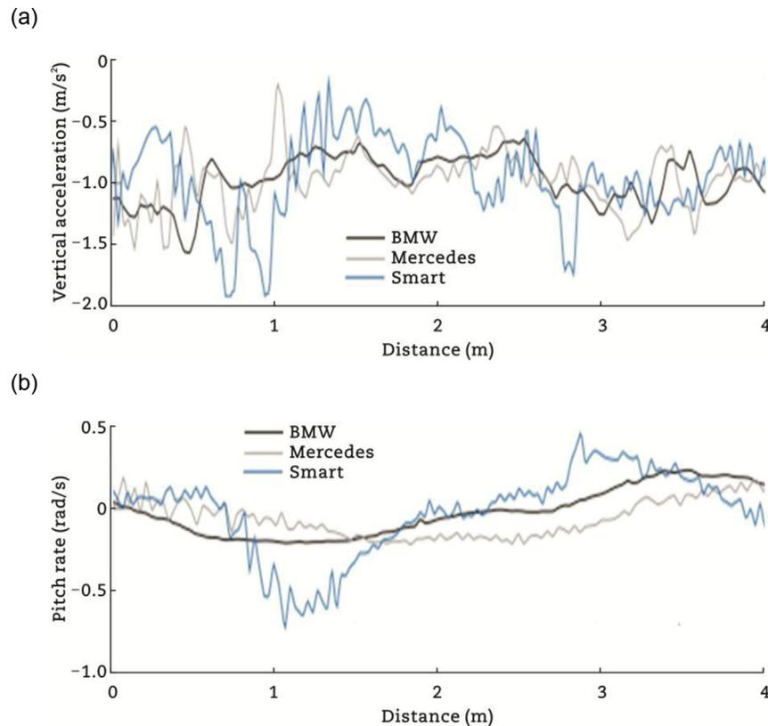
**Fig. 2 – Raw data of three vehicles driving over a pothole with a velocity of 7.5 m/s. (a) Vertical acceleration. (b) Pitch rate.**
