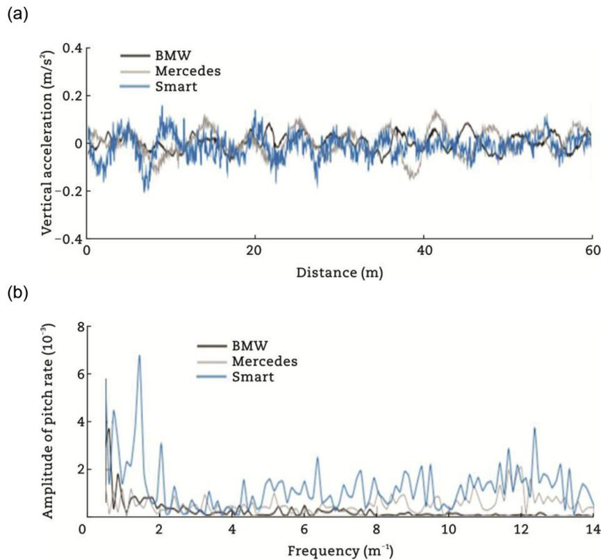
**Fig. 3 – Data of three different vehicles driving over the same segment of a rough road at about 7.5 m/s. (a) Vertical acceleration. (b) Amplitude of pitch rate.**
