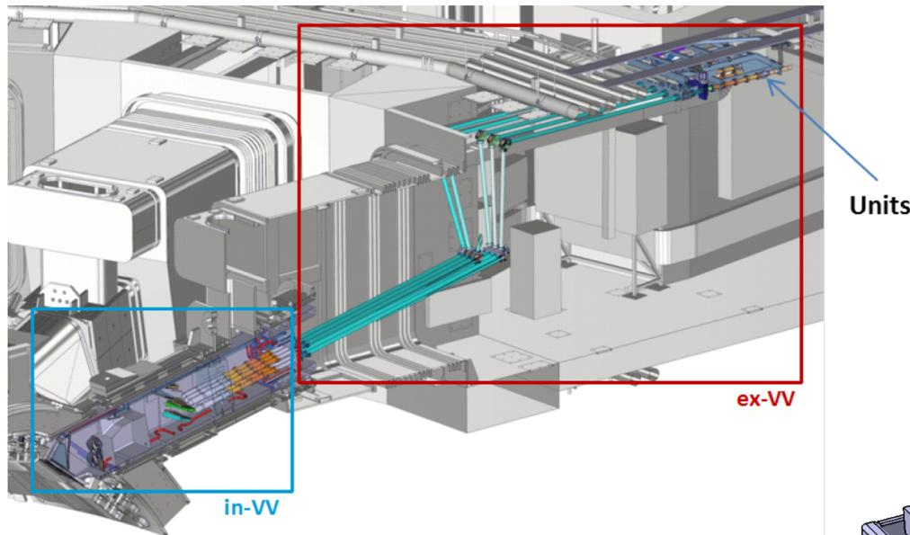
The Upper Launcher consists of an assembly of ex-vessel waveguides and an in-vessel port plug.
