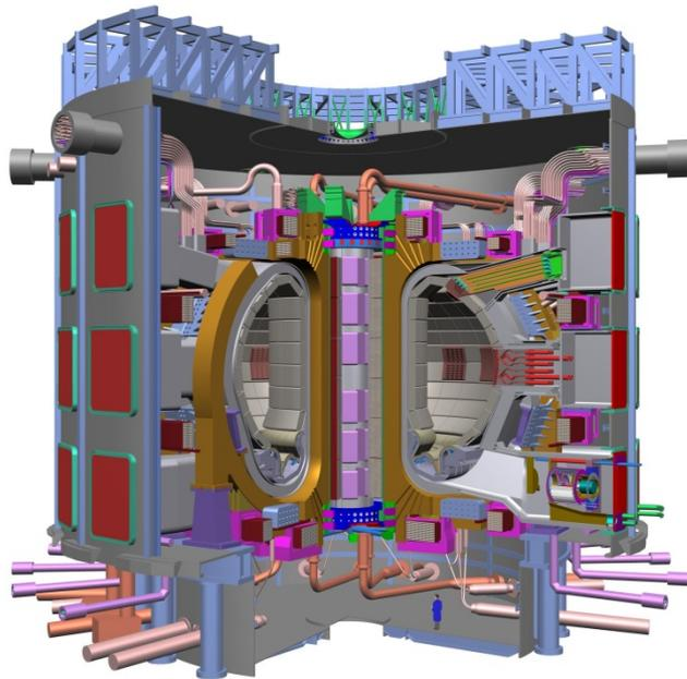
ITER is an experimental machine based on “tokamak” concept and designed to prove the feasibility of fusion as a large-scale source of energy.
