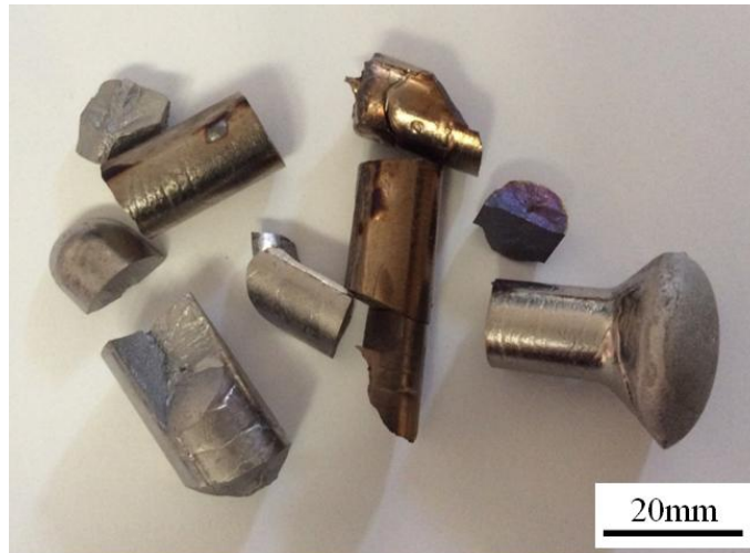
Figure 6.2: Rod of X5 after arc melting
