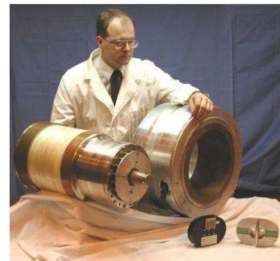
1990's – Westinghouse STC 1 MW, 20 K BSCCO Superconductor
