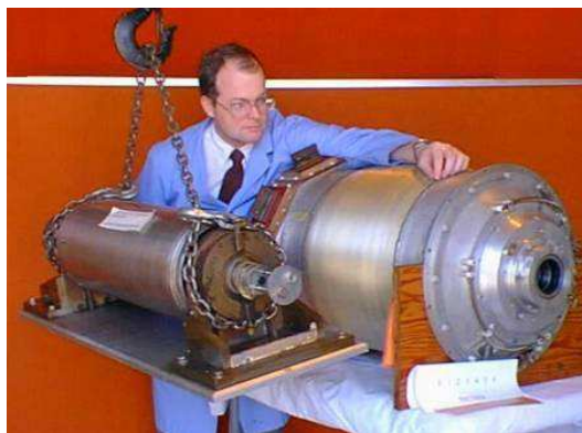
1970's - Westinghouse 5 MW, 4.5 K NbTi Superconductor
