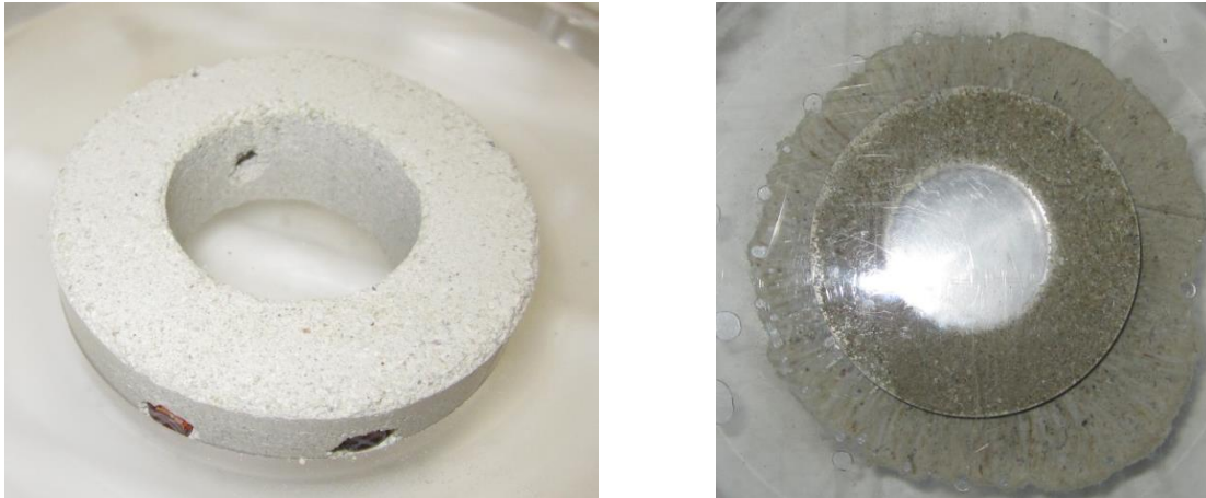
Figure 29: (left) Bentonite sample with holes on side of the ring containing filled glass vials. (right) Top view of the bentonite ring in the swelling stage.
