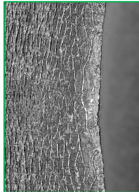
burst opening side, \approx 20 cracks/mm
