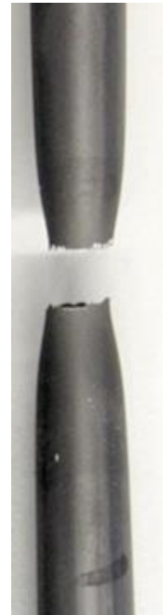
QL-3, clad #12 necking far away from burst region
