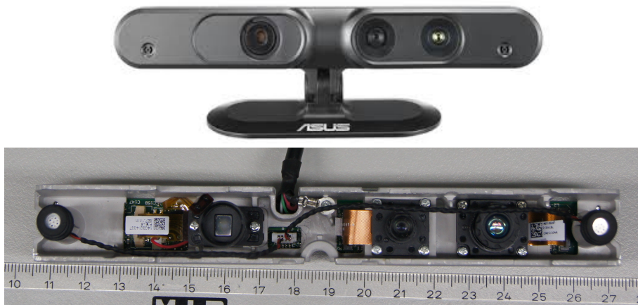
Figure 3.17.: ASUS Xtion, based on the same chip as Kinect v1 but in a compact form factor. It is the device that was finally installed in our MRD.
