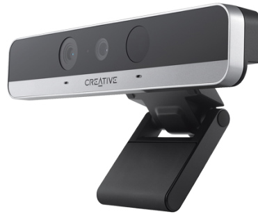
Figure 3.16.: Intel RealSense device. It is a projected pattern device also better suited for close range interactions.
