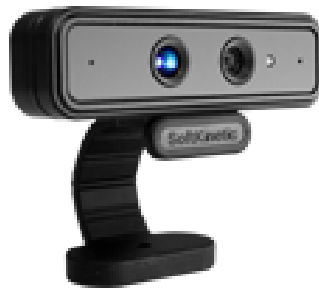
Figure 3.15.: The SoftKinetic development system is also a TOF camera, and it was also better suited for close range interaction tasks.
