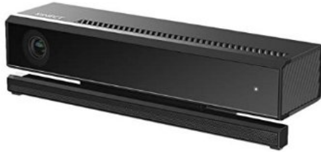
Figure 3.13.: Kinect v2 from Microsoft. It is the best depth camera currently available, however it is bulky, and requires a powerful PC just to capture the depth signal, thus it is not well suited to be integrated.
