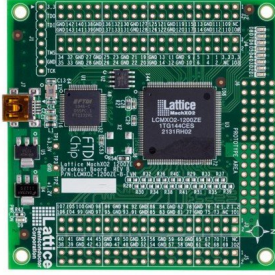
Figure 3.22.: MachXO2 development board. The MachXO is a FPGA marketed as a Complex Programmable Logic Device (CPLD).
