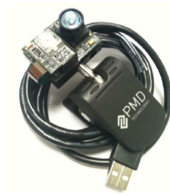
Figure 3.14.: The PMD NANO is a compact TOF device well suited for integration, but it is better suited for close range interaction tasks.
