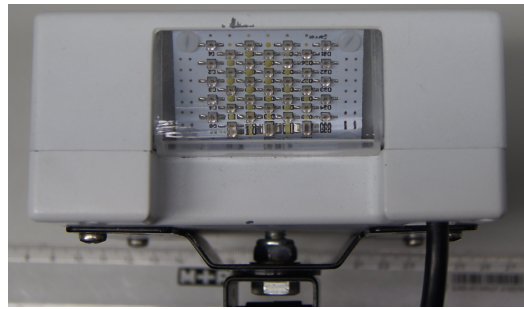
Figure 3.26.: Infrared illumination window on the MRD. It is tilted 30 degrees towards the ceiling.
