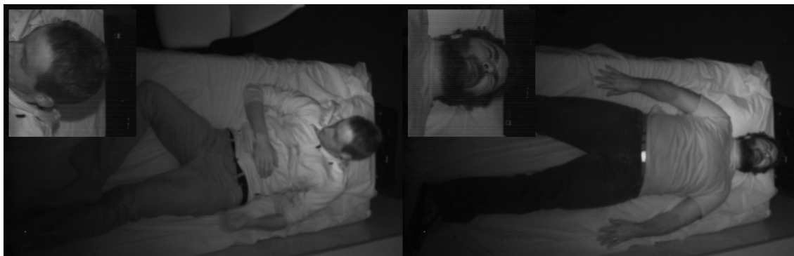
Figure 3.2.: Images from one of the stereo cameras and the face camera. Images from the face camera are more detailed and can be captured at 100 fps due to its reduced ROI. As the faces obtained from our device are rarely frontal, we must combine tracking and detection to aim the camera.
