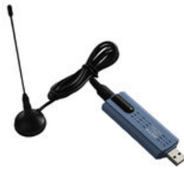
Figure 3.31.: TV Receiver used to debug the electrical emissions of the MRD.
