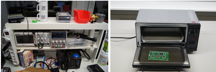
Figure 3.20.: Left: workbench we built to debug the problems with the camera board. Right: pizza oven used to resolder all delicate components.
