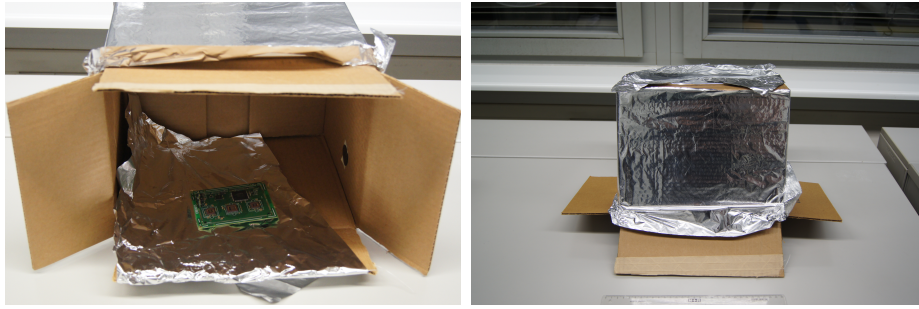
Figure 3.32.: We tested the device inside this box to avoid external EMC interferences. We latter used a microwave for improved isolation.
