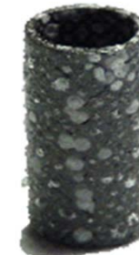
SiC-SiC f cladding after 64 h at 1600°C in steam
