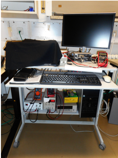
Fig. 4.11.: Photo of the complete calibration setup (left panel) including the readout computer and the power supply units. The positioning system with the sensor and beam pipe mock-up are covered in black tissue. The right panel shows a detailed photo of the power supply units.
