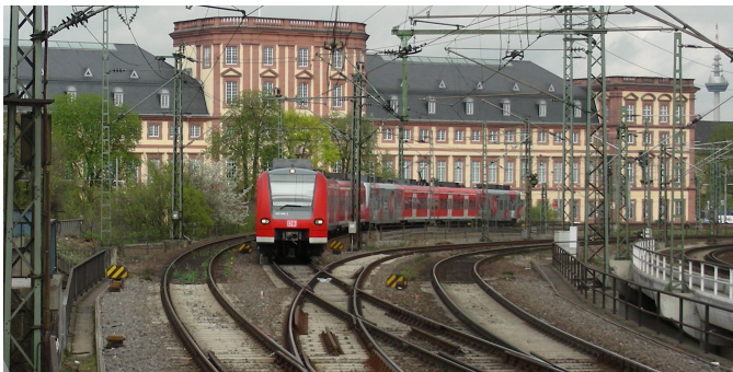
(b) Several tracks with a diamond crossing in front of the train.
