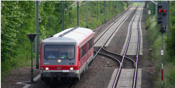
(a) Two parallel tracks that are connected by two single turnouts.
