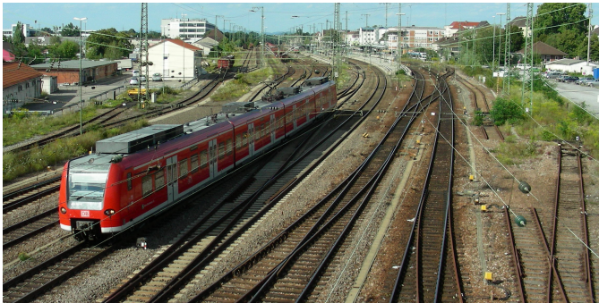
Figure 2.6: Exemplary scenario near a railway station with several tracks and single turnouts. The parallel tracks left and right of the railway vehicle will be within the detection area. Especially the tracks in the right part of the picture are too far away (photo by courtesy of Martin Lauer).
