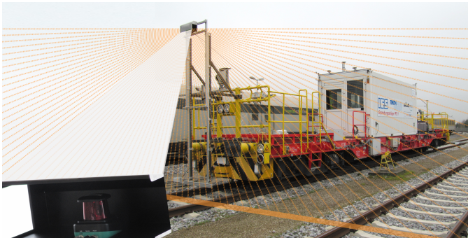
Figure 3.1: Experimental railway vehicle IFS 1. The lidar sensor (scale-up on the lower left side) is mounted vertically on the front. Thin orange lines represent selected laser beams which generate a profile of the environment.
