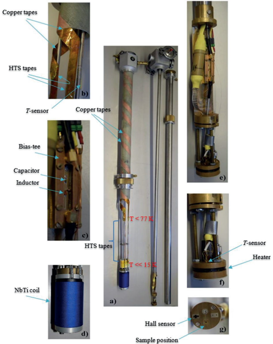
Figure 6.2: a) Variable temperature insert with a superconducting coil and vacuum sample rod. The vacuum sample rod is assembled in the dipstick with coil during operation. b) The stage of coupling of the copper and high-superconducting tapes. c) Embedded bias-tee d) Superconducting NbTi coil with central field up to 2 T at 4.2 K. e) Carrier board for electrical and optical components. f) Sample holder with embedded temperature sensor on the back side, heater and SMA fiber connector for back side illumination. g) View of top side of the holder with Hall effect sensor for control magnetic field.
