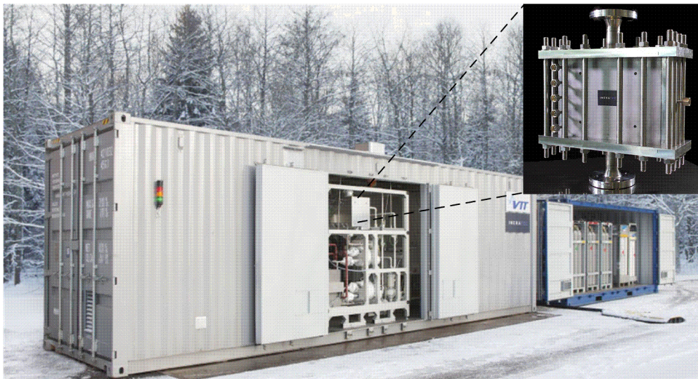
Figure 1–11 Containerized FTS plants (14 kg/d) built by INERATEC for VTT Technical Research Center of Finland [85, 86]
