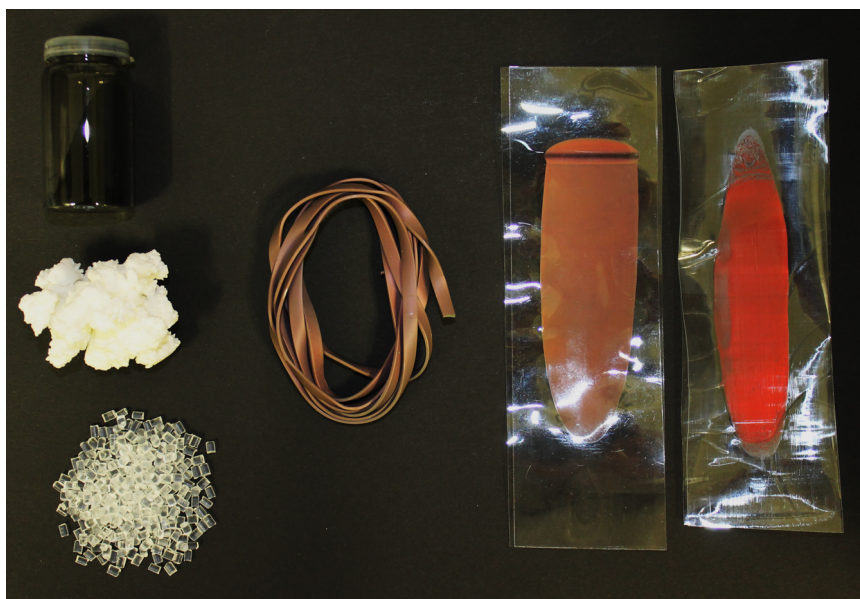
Figure 6.7: Materials and products at different stages of the fabrication process. A A small amount of carbon black (top) is extruded with coagulated PO particles (middle) and TFX granules (bottom) in various weight ratios (here 15 wt%) to colorful strings with a 5 \times 1 \text{ mm}^2 profile (B). The compound is spread between two PET-sheets (C) and subsequently sheared over a hot edge to order the PO particles and enhance the color (D).
