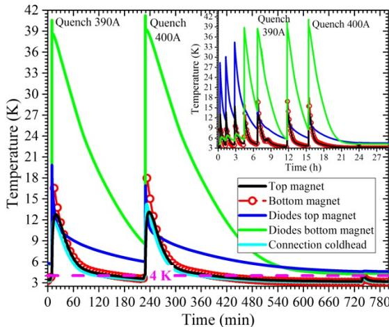
Figure 6: Temperature behavior during two quenches near the operating current. The inset shows the complete quench series of cooldown 3.
