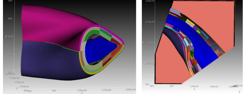
Converted HELIAS model in DAGMC representation including material layers, last closed flux surface (blue) and bounding box
