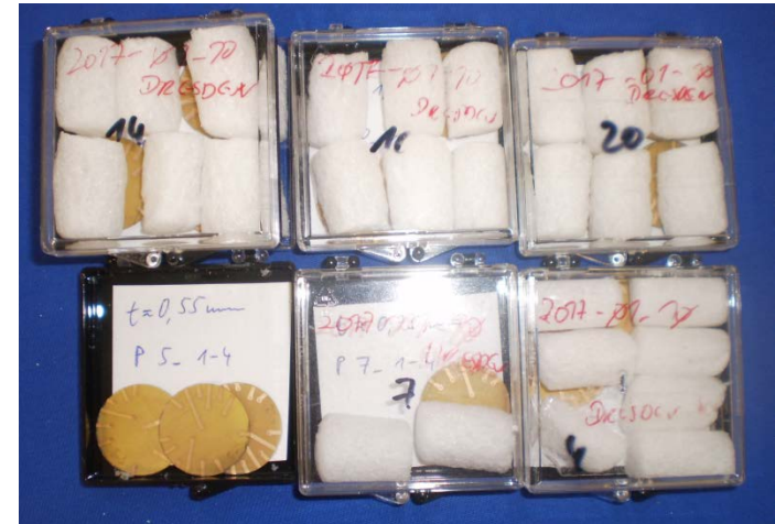
Produced 24 piezofibre discs from one batch of fibres and moulding
