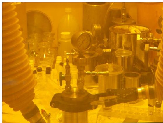
**Fig. 6:** Autoclave for dissolution experiments, loaded with a steel specimen, inside a shielded box. The gas-collecting cylinder is not yet connected to the autoclave.
