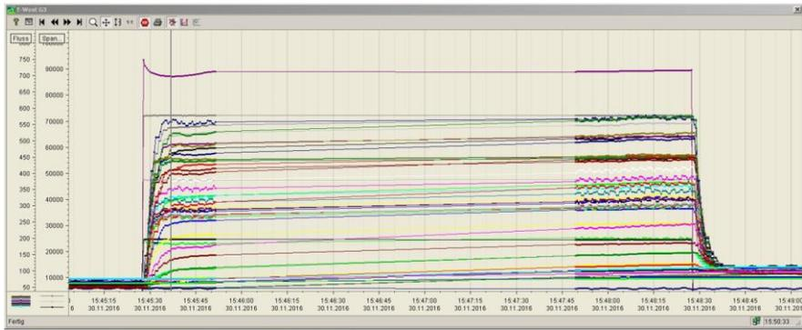
Fig. 1.2.22: Collector's thermocouple temperature and  $I_{beam}$  during a 180 sec pulse.
