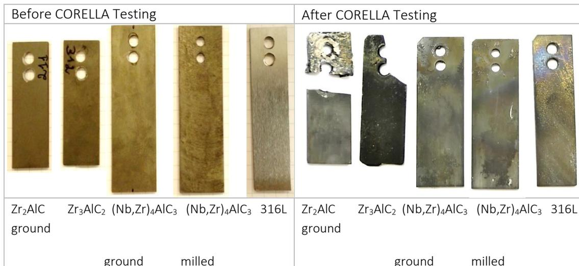
Fig. 3.2.1: Photos of specimens before and after 1000h erosion corrosion test at 500°C.
