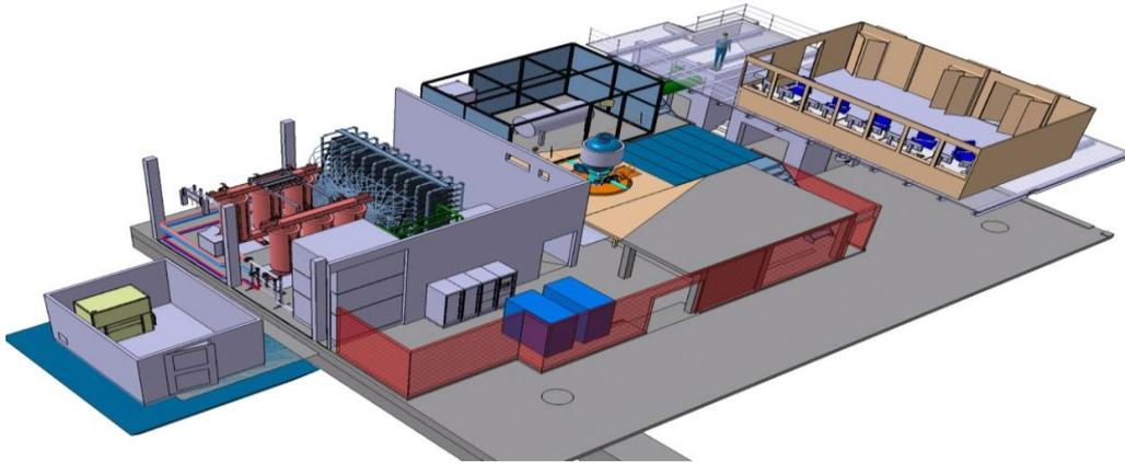
**Fig. 1.6.1:** CAD view of FULGOR installation including control room.
