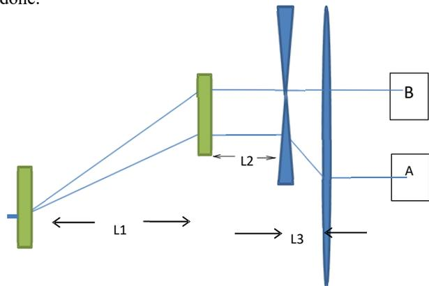
Figure 4: Modification of the concept shown in Fig. 2 for linearizing the pathlength with additional magnets (one out of several possibilities).
