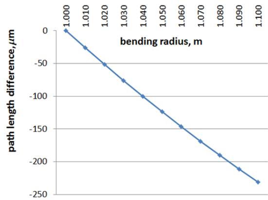
Figure 3: Path length differences in  $\mu m$  for particles with an energy difference of up to 10 % energy deviation bent by a 20 cm 1T magnet. Beam energy: 300 to 330 MeV. This curve shows the nonlinearities in the length already described in equation (2). Since the trajectories are locally separated the trajectory length can be corrected by additional magnets (not discussed in this paper). Figure 4 shows one possibility (among several other) how this can be done.
