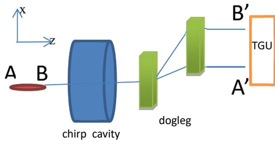
Figure 2: Concept for producing coherent radiation with a TGU. If the chirp and the dogleg is designed so that all electrons arrive at the same time ( $A-A' = B-B'$ ) at the surface of the TGU the emitted radiation is monochromatic. If the length of the incoming particle beam entering the TGU is shorter than the laser wavelength the preferred laser concept is described by A, otherwise by B.
