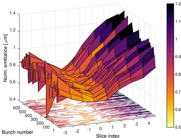
Figure 7: Normalised horizontal slice emittance measured along the bunch train (in steps of 10 bunch numbers). Slice index 0 corresponds to the central slice with maximum bunch current.
