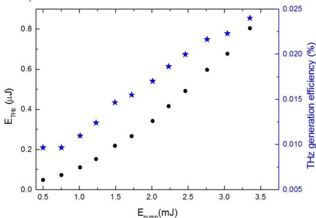
Figure 2: THz pulse energy (black dots) and conversion efficiency (blue stars) as a function of pump energy.
