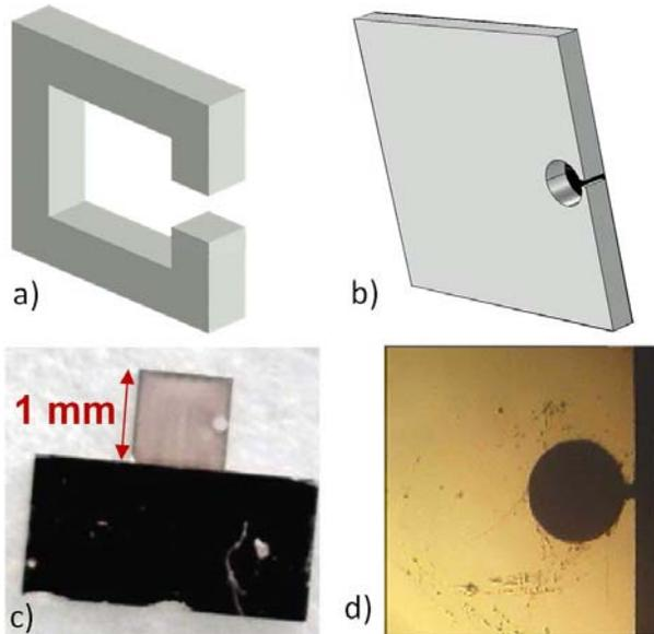
Figure 4: a) “Classical” SRR [5] with gap dimensions of 20  $\mu\text{m}$  (height) x 20  $\mu\text{m}$  (width) x 20  $\mu\text{m}$  (length), b) manufacturing design with increased gap length / plate thickness of 20  $\mu\text{m}$  x 20  $\mu\text{m}$  x 80  $\mu\text{m}$ , c) and d) images of the prototype SRR made from glass with gold coating.
