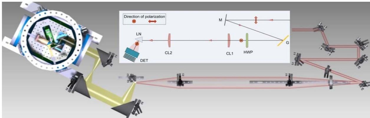
Figure 1: Layout of the THz source at FLUTE (shown in red and schematically in the inset). M: dielectric mirror; G: reflection grating; HWP:  $\lambda/2$  retardation plate; CL1: plane convex cylindrical lens ( $f = 421$  mm); CL2: plane convex cylindrical lens ( $f = 250$  mm); LN: MgO doped stoichiometric LiNbO<sub>3</sub> prism. The THz-transport to the SRR in the vacuum chamber is also shown (yellow beam path).
