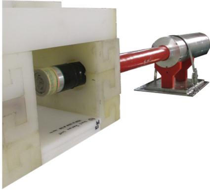
**Fig. 3:** Experimental setup showing the NE213 detector. The picture was taken before the rear side of the PE house was closed. The scintillator position indicated by the yellow/green tape is inside the house while the light guide inside of the red tube and the adjacent photomultiplier in the metallic cylinder is located outside of the housing.
