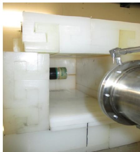
*Fig. 2: Experimental setup at the end of the beam line. The target was located in the beam line visible on the right; behind the beam line a polyethylene housing was mounted (white bricks) in which the NE213 detector (the scintillator position is indicated by the yellow/green tape) was placed.*
