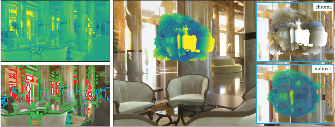
Figure 10.4: Top Left: false-color rendering . Bottom Left: illuminance contour lines . Center and Right: spherical plots visualizing the flow of light above a sitting area . Insets: chroma coloring of the plot and filtering out peaks by visualizing only indirect lighting .
