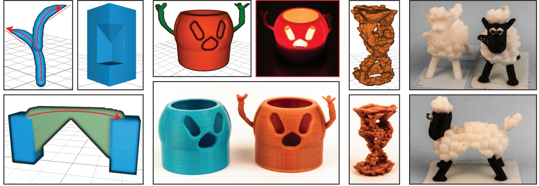
Figure 5.3: Left: examples of an add-trim stroke, a remove-preserve operation where a cube is subtracted from a pillar, and an add-grow stroke which automatically creates a bridge underneath. Center: the PUMPKIN model can be used as a tea-light holder. Center Right: a more intricate sculpture. Right: more prints of the SHAUN model. All shapes are support-free.
