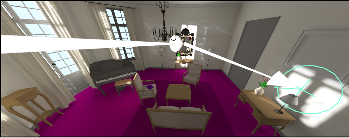
Figure 8.6: The light path tool is used to inspect where the caustic is coming from, and reveals that it is a reflection of the sunlight from a mirror at the back wall.
