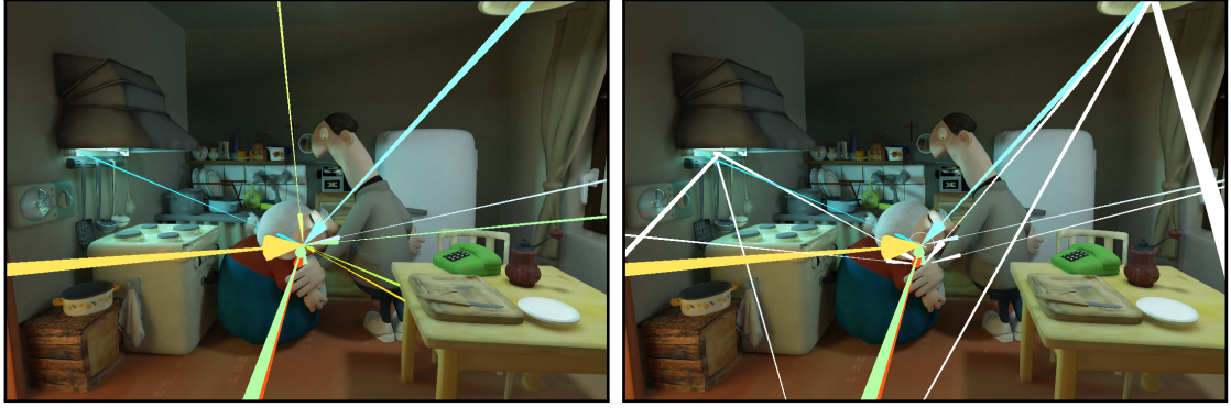
Figure 8.7: The light path tool is prone to create visual clutter. This phenomenon amplifies for multiple light path bounces. This is why we prune paths according to a cut-off threshold \epsilon . Left: single-segmented paths with \epsilon = 0.1 . Right: one additional bounce with \epsilon = 0.16 .
