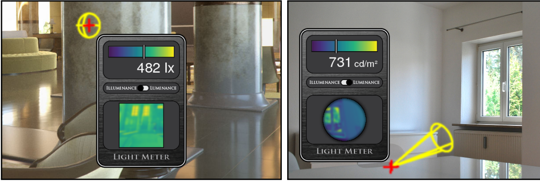
Figure 10.6: A virtual light meter allows to measure photometric quantities.
