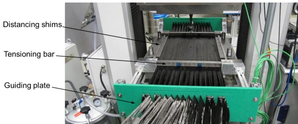
Figure 5.8: Permeability mold with carbon fiber roving stack
