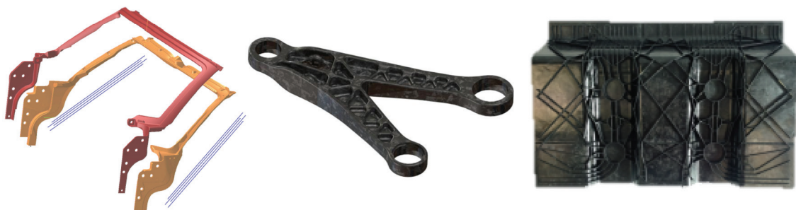
Figure 2.7: Structural components made of CoDicoFRTS left: Windshield surround [22] center: Suspension arm [21] right: Subfloor structure [76]
