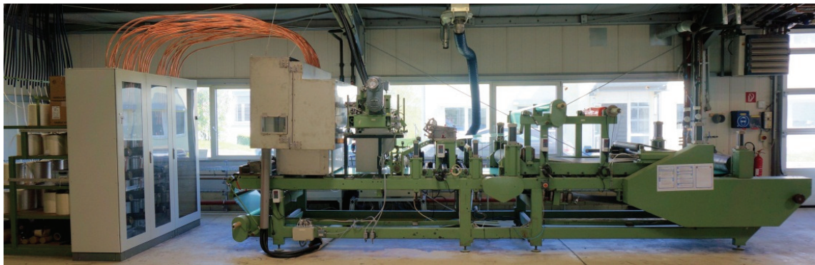
Figure 4.2: Modified flat conveyor plant HM-LB-800
