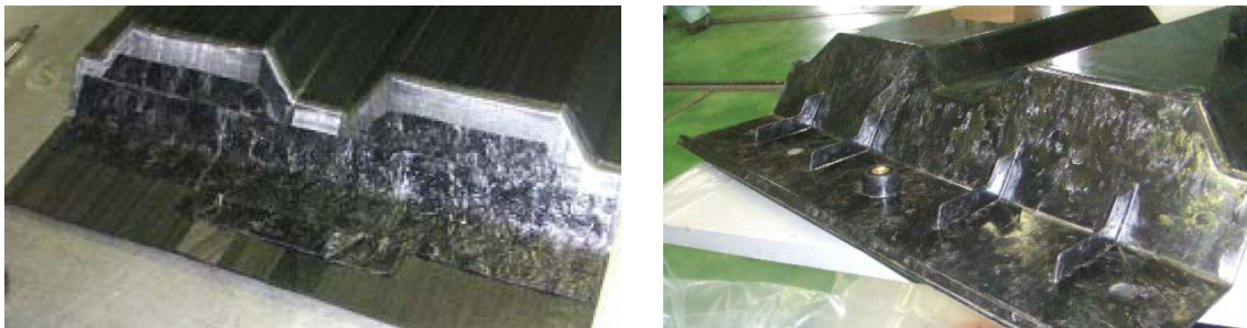
Figure 2.8: CF-SMC mold coverage before co-molding and final part [19]
