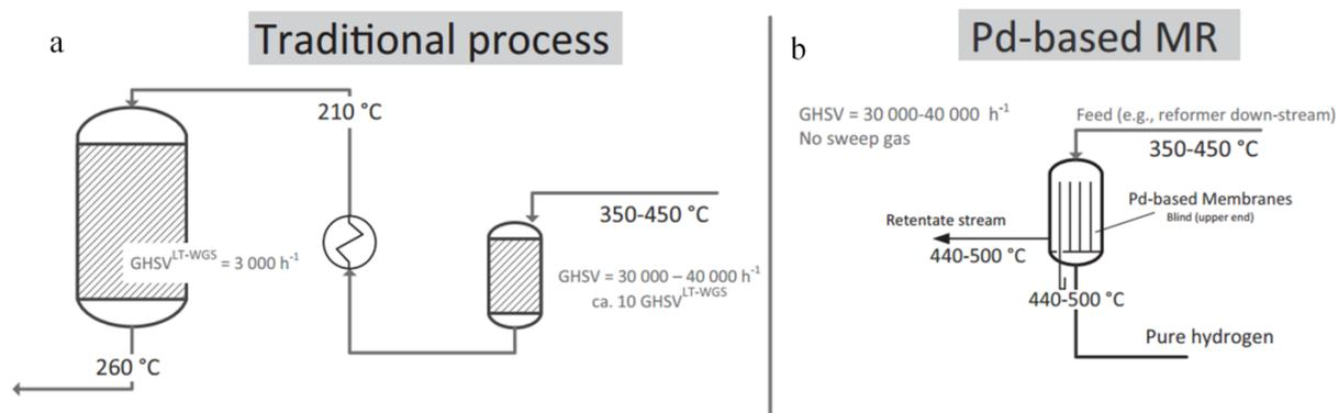
Figure 1.7: Schematic drawing of “traditional reactor process (TR)” (a) and “Pd-based membrane reactor (MR)” (b) for WGS reactions (the values for temperature and GHSV indicate a typical operation parameter) with permission from [69].
