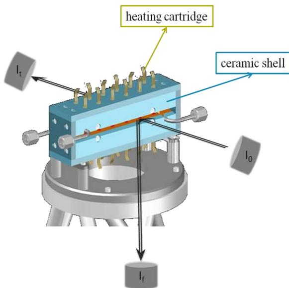
Figure 3.5: Schematic drawing of the XAS set-up using the WGS microreactor. The intensities of the incoming ( $I_0$ ) and transmitted ( $I_1$ ) monochromatic beam are measured in transmission mode. The intensity of a specific x-ray fluorescence line ( $I_f$ ) is detected in fluorescence mode.
