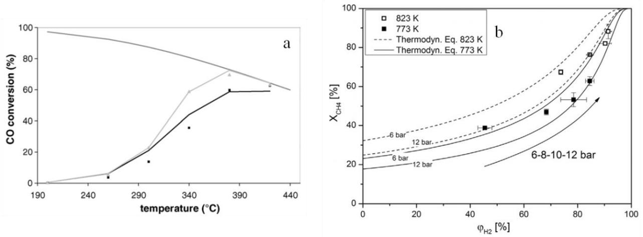
Figure 1.10: (a) Comparison between stainless steel microchannels (grey) coated with Pt/CeO<sub>2</sub>/Al<sub>2</sub>O<sub>3</sub> catalyst (containing 1.7 wt.% Pt, 10.7 wt.% CeO<sub>2</sub>) and as powder samples (black); the symbols represent experimental data, the lines model calculations, with permission from [78]. (b) Methane conversion as a function of hydrogen recovery for an integrated steam methane membrane micro channel reformer, reprinted with permission from [76].
