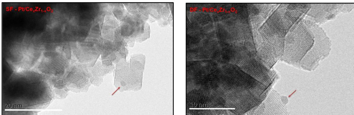
Figure A.7: TEM images of  $Ce_xZr_{1-x}O_2$  supported Pt nanoparticles made by single flame (SF), and double flame (DF) spray pyrolysis, recorded at Dalian Institute of Chemical Physic (DICP), Chinese Academy of Sciences (CAS) in Dalian/China.
