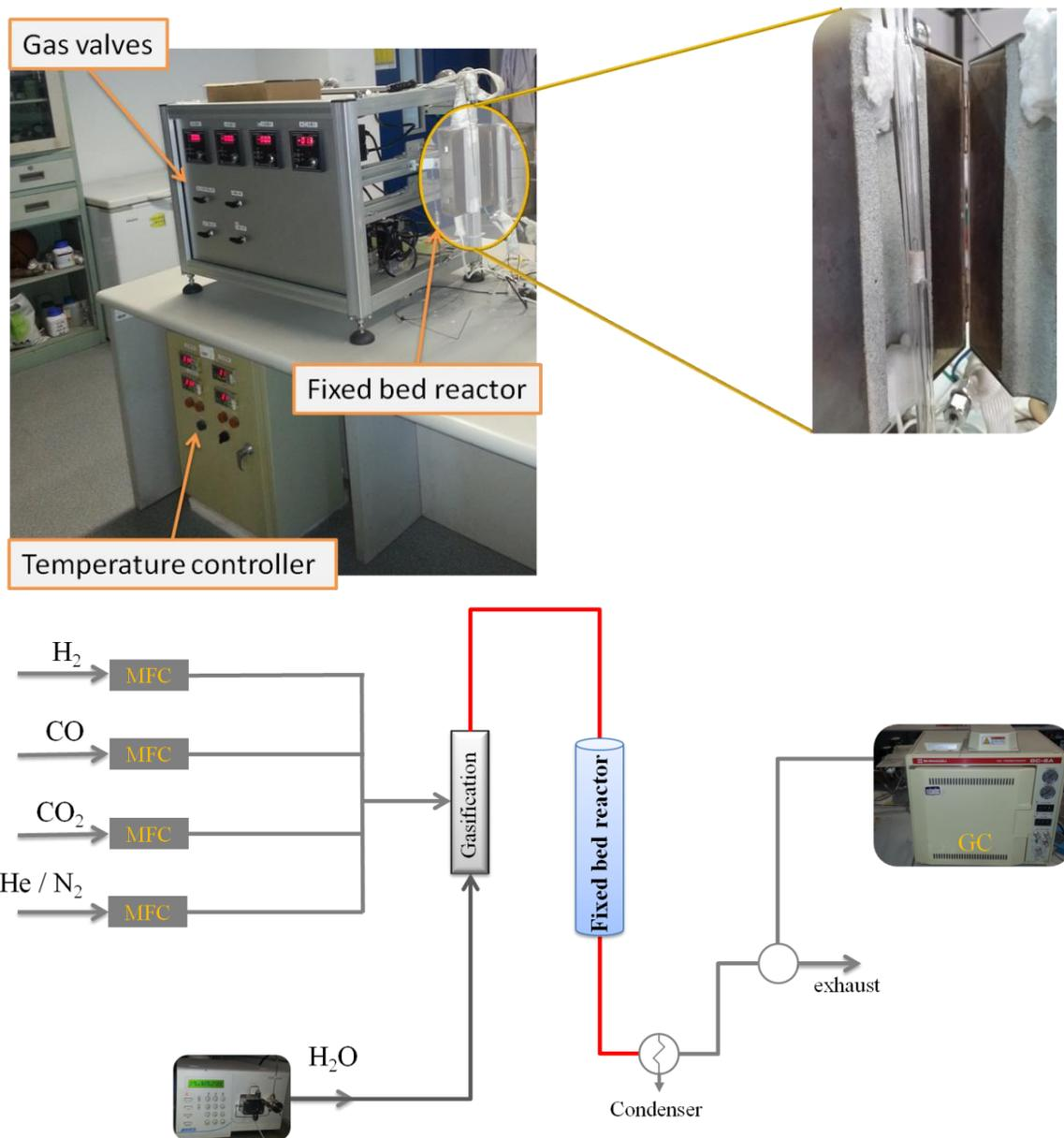
Figure 3.7: Photograph (top) and a schematic drawing (bottom) of activity test set-up for water gas shift reactions at Dalian Institute of Chemical Physics (DICP, China).
