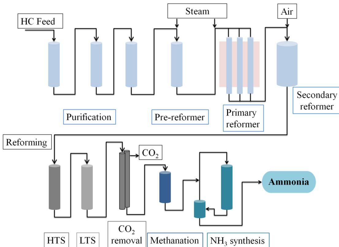
Figure 1.1: Industrial application of ammonia production for the Haber-Bosch process (adapted from [11]).
