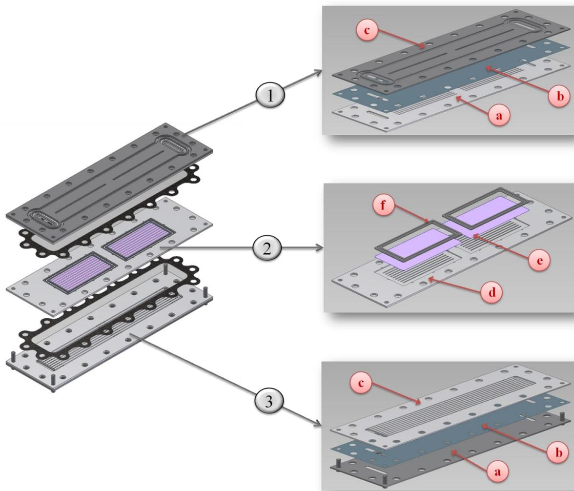
Figure 3.3: Micro-structured membrane reactor for *in situ* XAS studies under WGS reaction conditions. Sub-assembly 1 (retentate): channels for catalysts and feed gas, X-ray window. Sub-assembly 2: membrane for hydrogen separation. Sub-assembly 3 (permeate): channels for swap gas for hydrogen, X-ray window.
