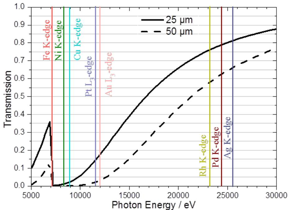
Figure 3.4: Calculated X-ray transmission through Fe based window materials (thickness of one window  $\rightarrow$  25  $\mu\text{m}$  and two windows  $\rightarrow$  50  $\mu\text{m}$ ) as a function of photon energy. The adsorption edges of different elements illustrated in relation to the transmission of X-rays.
