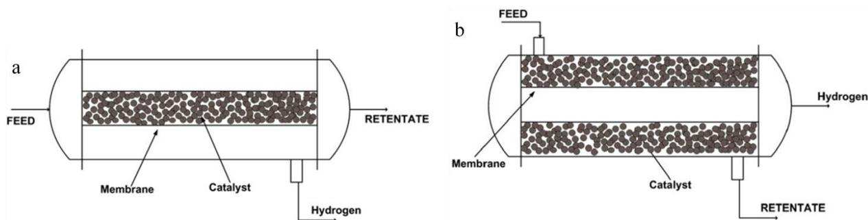
Figure 1.9: Typical packed bed membrane reactors: (a) catalysts in tube and (b) catalyst in shell, with permission from [71]. The retentate is the part of the feed that does not pass through the membrane whereas the permeate contains the species passing through the membrane.
