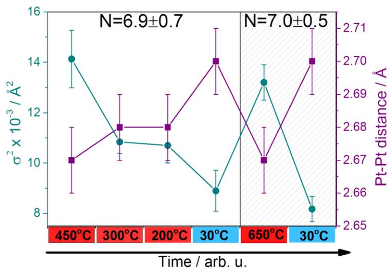
Figure A.3: Temperature-dependent Pt-Pt-bond length and Debye-Waller-Factor of 3.7 wt.% Pt/CeO<sub>2</sub> catalyst.
