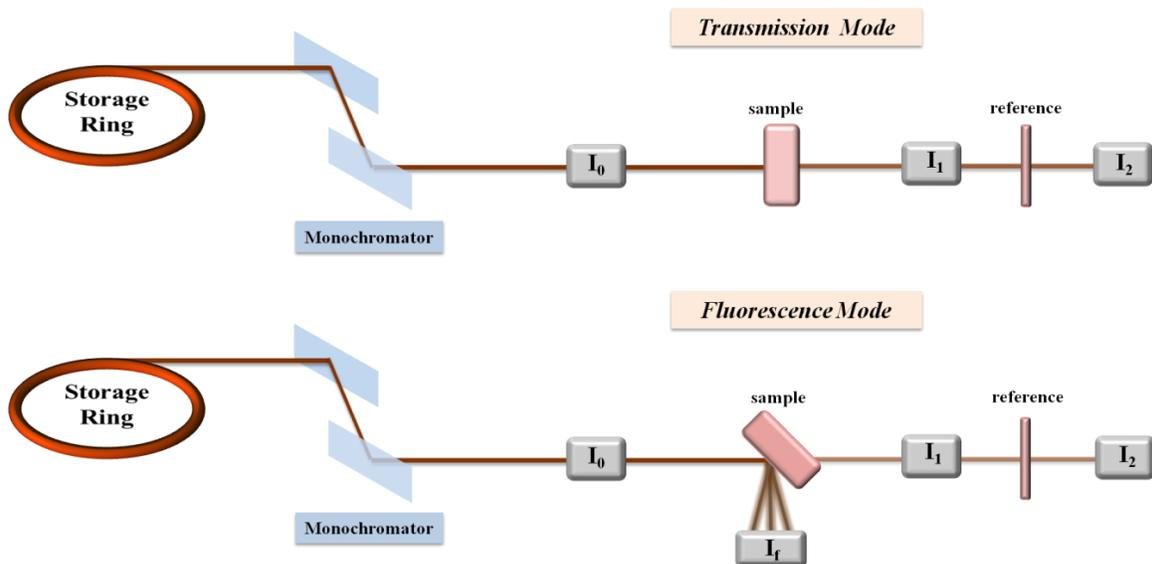
Figure 1.14: Experimental set-up for XAS measurements in transmission (top) and in fluorescence (bottom) mode ( $I_0$ : incoming intensity,  $I_1$  and  $I_2$ : transmitted intensity, recorded from the first, second and third ionization chambers;  $I_f$ : intensity of fluorescence radiation, recorded from fluorescence detector).
