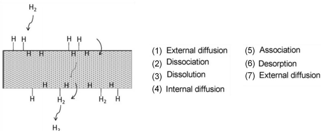
Figure 1.8: Solution diffusion mechanism of hydrogen permeation through a palladium membrane reprinted with permission from [72].
