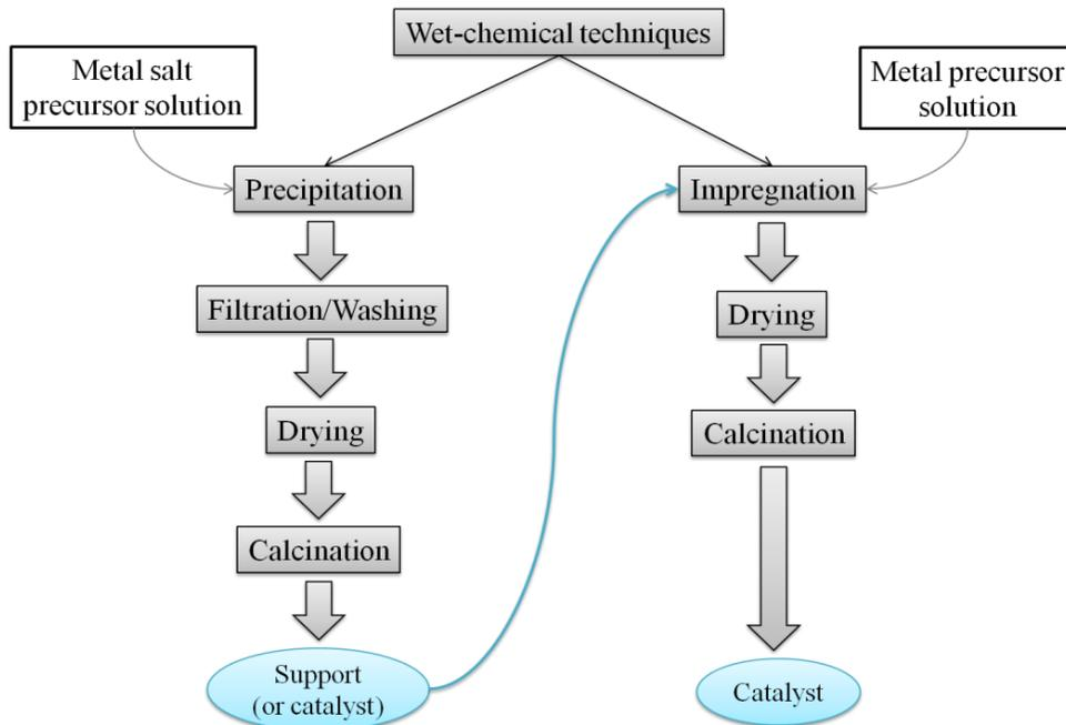
Figure 1.11: Preparation routes for technical catalysts (adapted from [80]).
