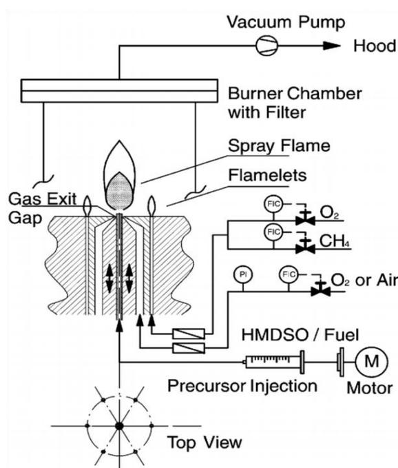
Figure 1.12: FSP set-up with an air-assisted nozzle and  $\text{CH}_4/\text{O}_2$  supply for the supporting flames, nanoparticles on a filter are collected with the aid of a vacuum pump with permission from [90].
