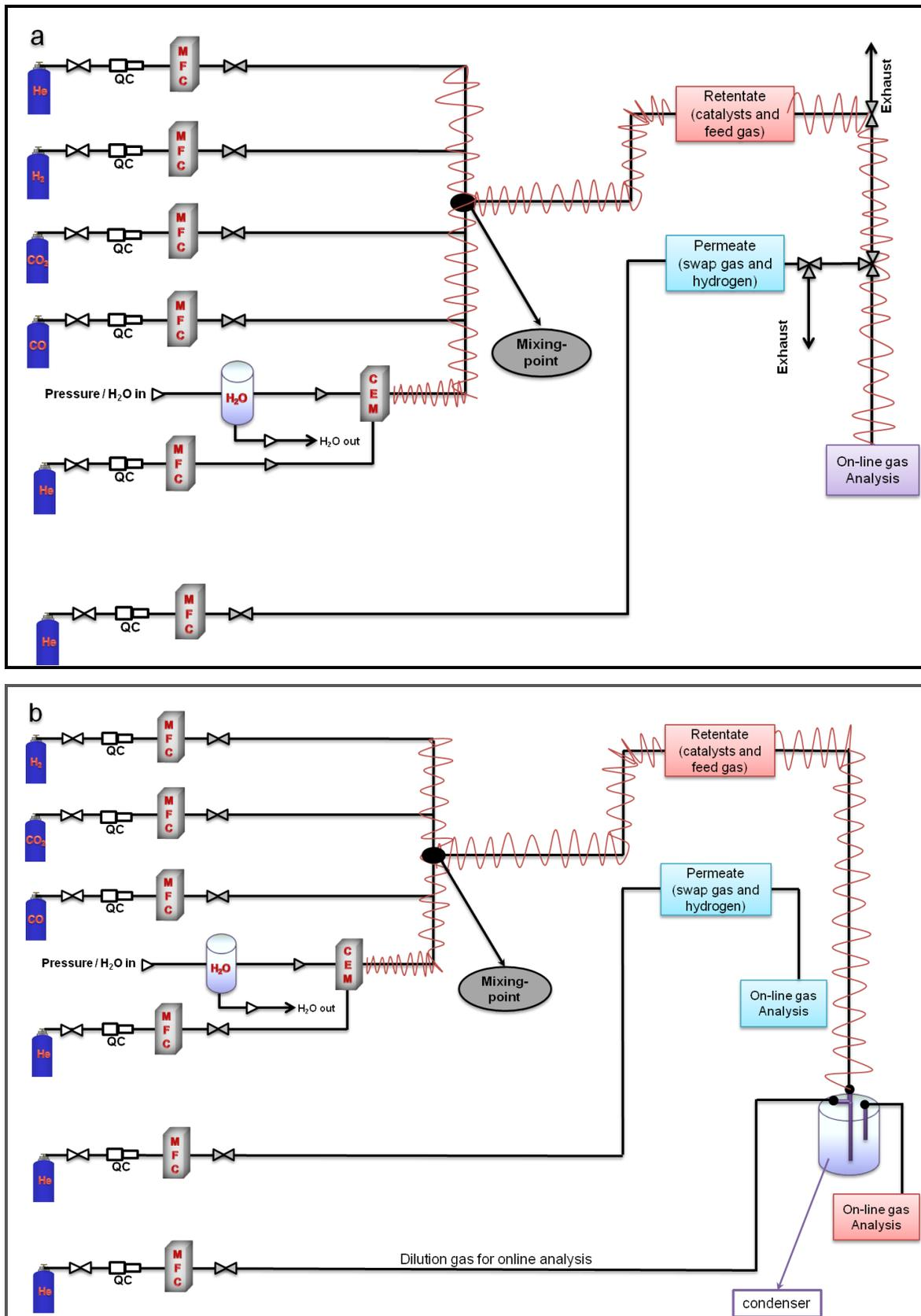
Figure 3.6: Gas dosing and water evaporation control system: (a) first version, (b) upgraded version
