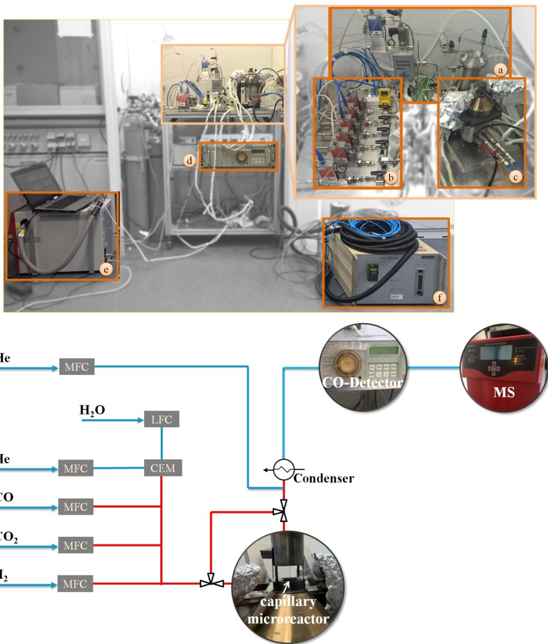
Figure 3.8: Photograph (top) and a schematic drawing (bottom) of the set-up for WGS activity test. Liquid Delivery System and controlled evaporation and mixing (a), mass flow controllers (b), gas blower (c), CO detector (d), mass spectrometer (e) and temperature controller for the gas blower (f).
