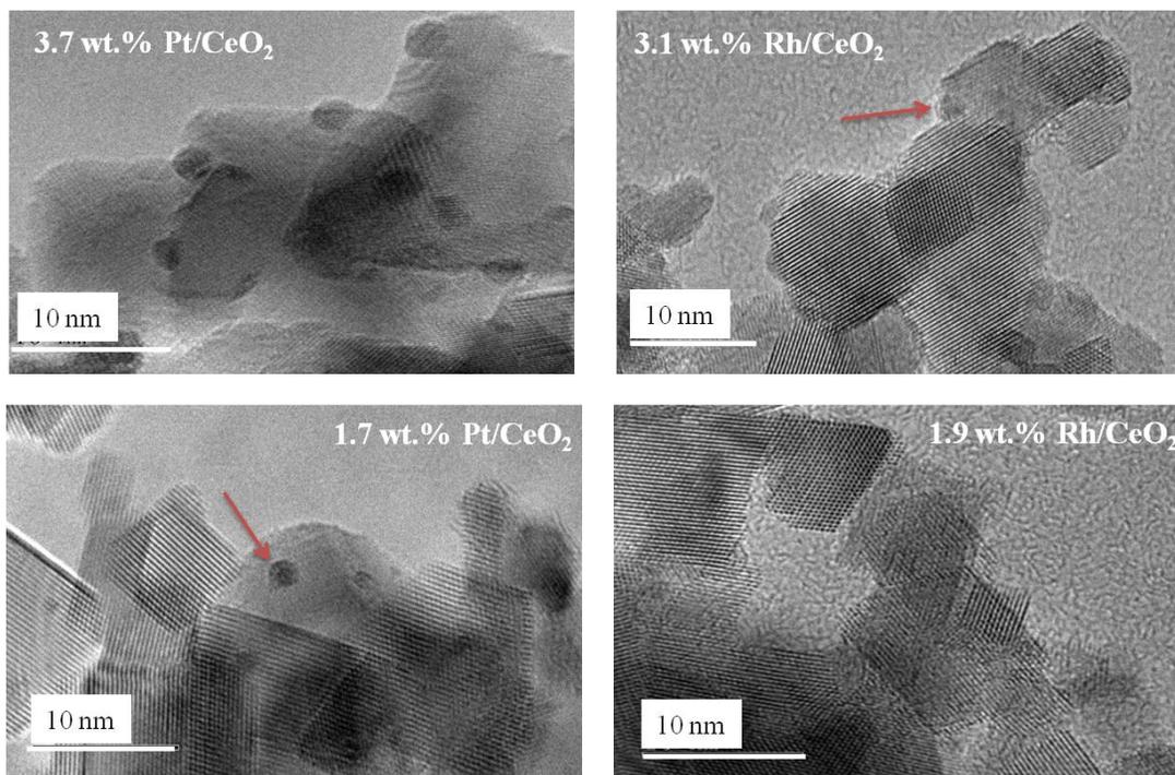
Figure A.1: TEM images of ceria supported noble metal catalysts: 3.7 wt.% Pt/CeO<sub>2</sub>, 3.1 wt.% Rh/CeO<sub>2</sub>, 1.7 wt.% Pt/CeO<sub>2</sub>, and 1.9 wt.% Rh/CeO<sub>2</sub> before water gas shift reaction (fresh samples). TEM images recorded at Dalian Institute of Chemical Physic (DICP), Chinese Academy of Sciences (CAS) in Dalian/China.
