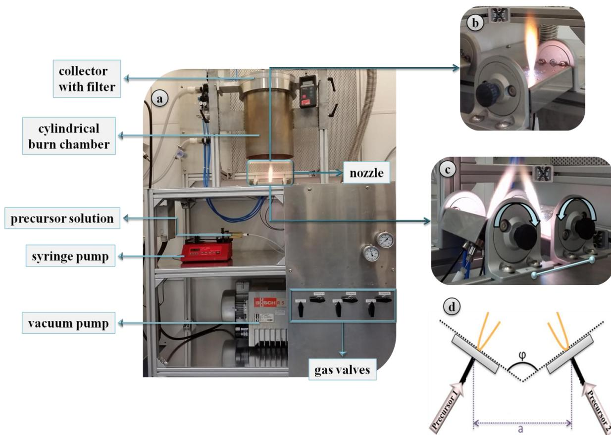
Figure 3.1: (a) Photograph of the FSP set-up at Karlsruhe Institute of Technology (KIT) with description of the different components. (b) Photograph of single flame spray pyrolysis and (c) double flame spray pyrolysis geometry. (d) Schematic drawing of the DFSP set up showing the angle  $\phi$  between the two nozzles and the inter-nozzle distance  $a$  between each nozzle center.
