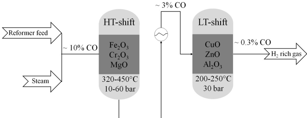
Figure 1.3: Two step industrial water-gas shift setup.
