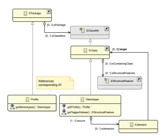
**Figure 4.14.:** The metamodel of EMF Profiles extends metaclasses of the metamodel of EMF. This extension enables a Profile to reference its corresponding AT and to contain Stereotypes. A Stereotype contains tagged values (realized as EStructuralFeatures) and extends metaclasses (EClasses) that are referenced via contained Extensions.
