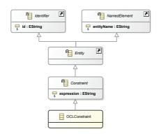
**Figure 4.12.:** The abstract metaclass Constraint inherits from Entity. The metaclass OCLConstraint realizes a concrete Constraint.
