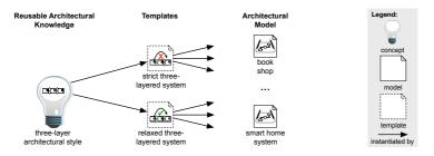
**Figure 2.10.:** Capturing variants of reusable architectural knowledge via templates that can be instantiated by architectural models (based on [Rie03]).
