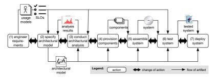
**Figure 2.12.:** Development process with integrated architectural analysis (based on [KH06]).
