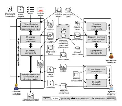
**Figure 2.13.:** Software architects specify an architectural model; component developers may provision components by implementing them anew; system deployers specify the allocation of the system to resources (based on [KH06]).
