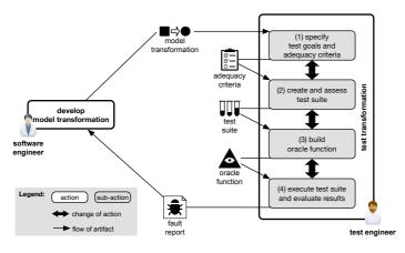
**Figure 2.9.:** Test engineers systematically test model transformations provided by software engineers.
