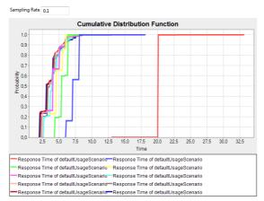
From left to right, the illustrated measurement belong to hard disk drive processing rates of 100, 90, ..., and 10 workunits. Here, we see that a hard disc processing rate of 20 workunits (dark blue values) already improves the response times to a great extend. The corresponding pie chart diagram of the hard disc utilization is shown below.
