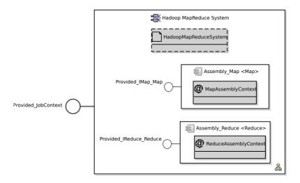
**Figure C.17.:** PCM system created by the default AT instance of the Hadoop MapReduce AT.
