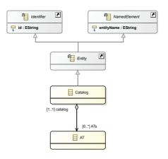
Figure 4.9.: The metaclass Catalog inherits from Entity and contains a set of ATs.
