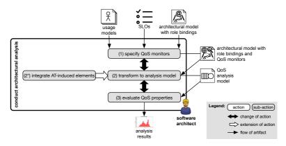
**Figure 4.3.:** AT-induced elements are automatically integrated during the transformation of an architectural model to a QoS analysis model.
