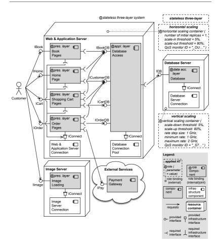
Figure C.12.: ATs for elasticity and cost-efficiency applied to the CloudStore model.
