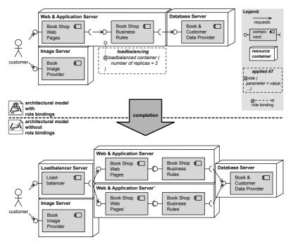
**Figure 4.4.:** A completion integrates elements induced by the loadbalancing AT into the book shop's architectural model, which defines the semantics of the bound role.
