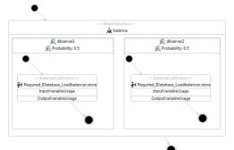
2. Next, we compose a new system by including the load balancer. For this, add the loadbalancer to the system diagram via a new »AssemblyContext«. As we have two databases now, we also add a database component via another new »AssemblyContext« and expand the assemblies name as well as the name of the second provided role of the load balancer by a »2« to ensure a unique naming. We connect the assemblies via »Assembly Connextors« such that we get a system diagram like shown below.
