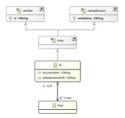
Figure 4.10.: The metaclass AT inherits from Entity and contains a set of roles.
