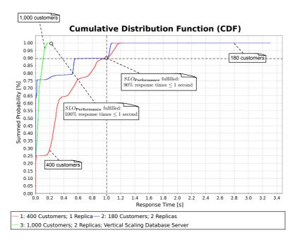
**Figure C.13.:** Cumulative distribution function of response times for different workloads and configurations of the modernized and migrated CloudStore (phase 2 and phase 3 of the CloudStore case study).
