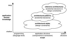
**Figure 2.5.:** Reusable architectural knowledge (cloud symbols) differs in scope (X-axis), application domain knowledge (Y-axis), and kinds of design decisions (parentheses within cloud symbols). The figure is based on [TMD09, p. 92].
