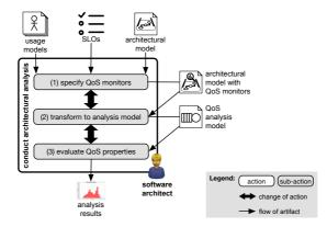
**Figure 2.14.:** Software architects conduct architectural analyses based on information from usage models, SLOs, and architectural models (based on [KH06]).
