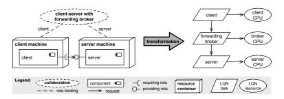
**Figure 6.5.:** A transformation from a UML model with a bound collaboration to a corresponding LQN model (based on [PW00]).
