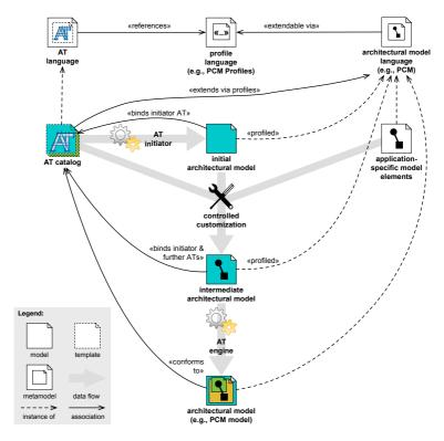
**Figure 4.6.:** Data flow of Architectural Templates (ATs). ATs are hybrid templates that combine initiator templates (for the creation of initial models and a controlled customization) and bound templates (for embedding further templates).
