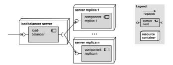
**Figure 2.6.:** The loadbalancing architectural pattern introduces a loadbalancer component to distribute workload.
