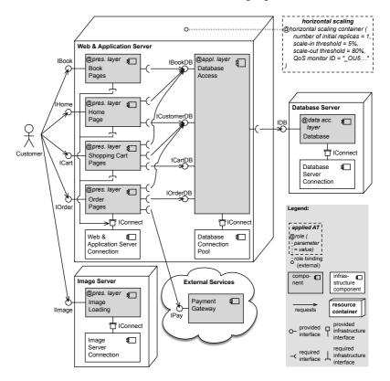
like shown in Figure C.10. Whenever the Web & Application Server is over-utilized, additional replicas are added and whenever the Web & Application Server is under-utilized, existing replicas are removed.
