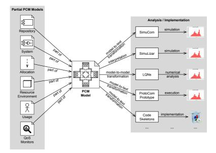
**Figure 2.16.:** The PCM includes partial, UML-like models for specifying QoS-relevant attributes of software systems (left). PCM models can then be analyzed and implemented in various tools (right).
