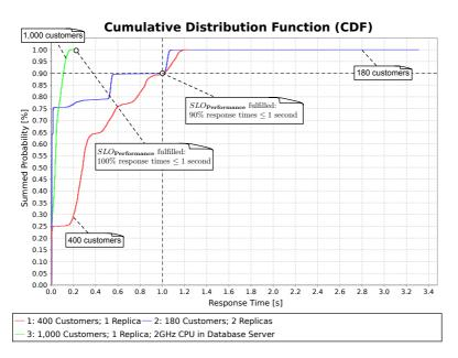
**Figure 3.6.:** Cumulative distribution function of response times for different workloads and configurations.
