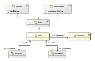
**Figure 4.11.:** The metaclass Role inherits from Entity, contains a set of constraints and an optional completion, and references a stereotype.
