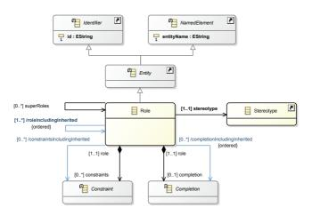
**Figure 4.16.:** The metaclass Role is extended by a new self-association superRoles that allows to specify inheritance relationships. Based on this relationship, the associations roleIncludingInherited, constraintsIncludingInherited, and completionIncludingInherited can be derived.
