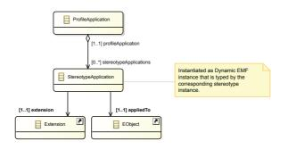
**Figure 4.15.:** A ProfileApplication contains stereotypeApplications. A StereotypeApplication applies a Stereotype (referenced via its Extension) to an EObject. Moreover, a StereotypeApplication is dynamically instantiated from a corresponding Stereotype instance, which allows StereotypeApplication to assign actual parameters to tagged values.
