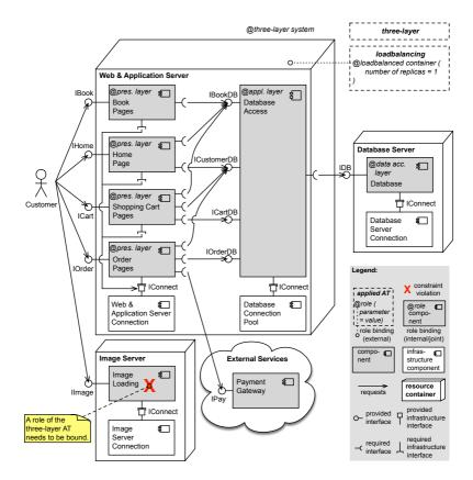
**Figure C.6.:** The three-layer and loadbalancing ATs applied to the CloudStore model (with constraint violation).
