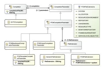
**Figure 4.13.:** The abstract metaclass Completion contains one or more parameters, which can be of different kinds. The metaclass QVTOCompletion realizes a concrete Completion.
