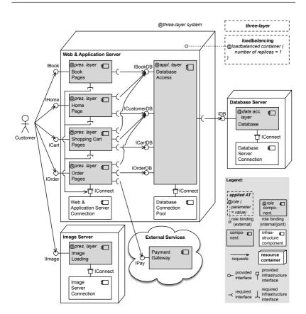
**Figure C.7.:** The three-layer and loadbalancing ATs applied to the CloudStore model (fixed version).
