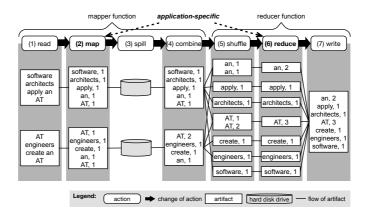
**Figure C.15.:** Performance-impacting actions of Hadoop's MapReduce processing pipeline exemplified for the WordCount application (based on [ZCL14]).
