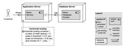
**Figure C.20.:** The horizontal scaling AT applied to the Znn.com model (based on [Rog16, Sec. 4.2.7]).
