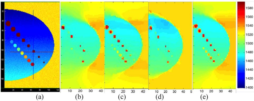
Figure 5: 3D simulation of a phantom (a) and reconstruction for 3D USCT II with different transducer distributions and parameters. 3D USCT II with 1 AP (b) and 16 AP (c), about  $15^\circ$  larger opening angles 1 AP (d) and 1 AP but uniform transducer distribution (e).
