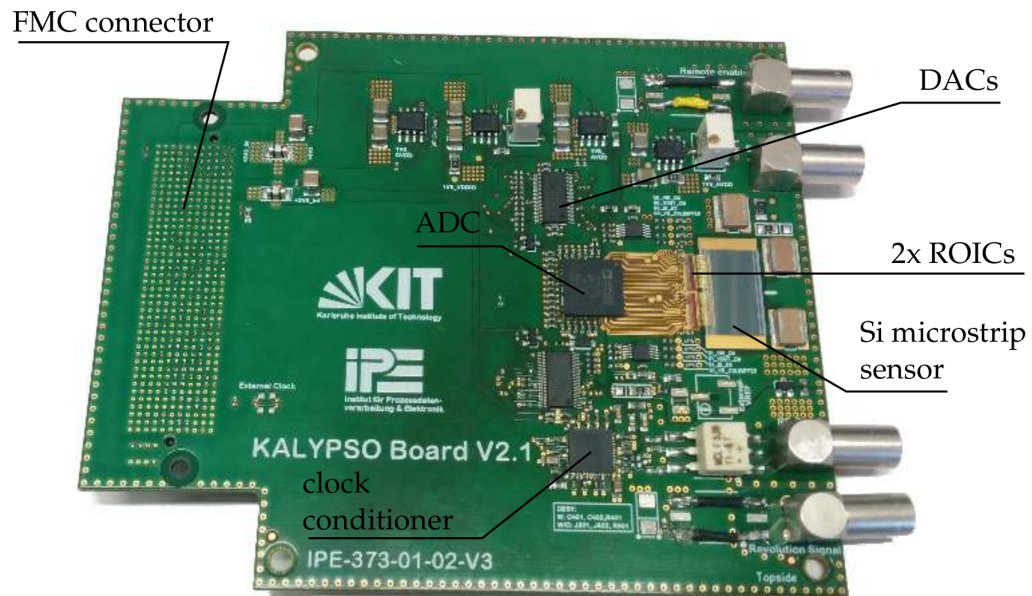
Figure 5.19. Picture of the KALYPSO detector board with Si sensor. DAC: Digital to Analog Converter, ADC: Analog to Digital Converter, ROIC: Readout Chip. Courtesy of L Rota
