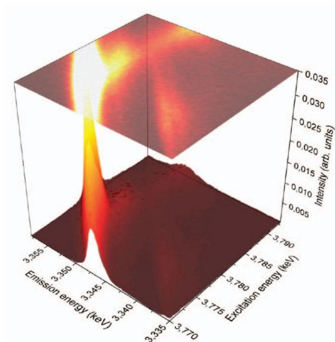
Figure 2: Pu M<sub>5</sub>-edge 3d4f RIXS of PuO<sub>2</sub>, recorded at the ACT station after commissioning of the high-resolution X-ray emission HRXES spectrometer.
