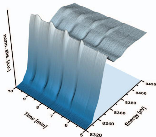
Figure 3: Structural changes in a Ni/Al<sub>2</sub>O<sub>3</sub> catalyst during hydrogen drop-outs representing the fluctuating availability of resources during the “Energiewende”; each time hydrogen is removed from a H<sub>2</sub>/CO<sub>2</sub> methanation gas mixture, the catalyst is slightly oxidized (cf. B. Mutz et al., *Catalysts* 7, 279 (2017)). Published under Creative Commons Attribution 3.0 DE License).
