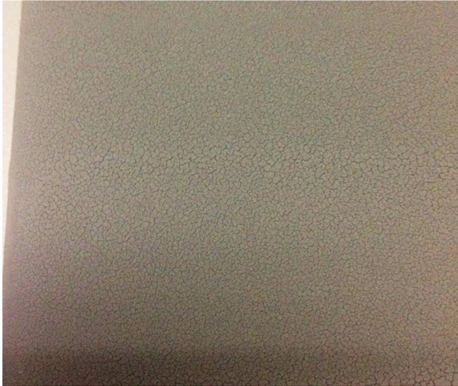
**Figure 57:** Top-down view of a sulfur cathode produced by water-slurry method; network of surface cracks. [61]
