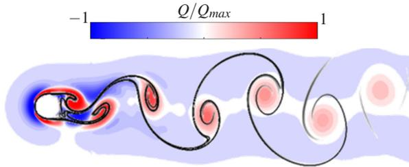
Figure A.1: Von Kármán vortex street:  $Q$ -criterion superimposed by an LCS determined by the backward FTLE.
