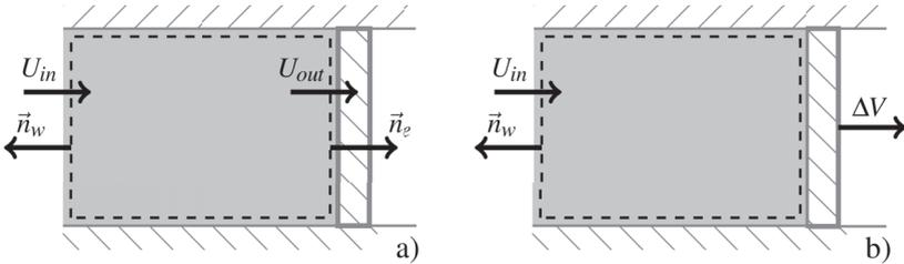
Figure 3.2: Two possibilities of defining a control volume in case of a moving boundary, where a) the volume change is taken into account via an outflow velocity,  $U_{out}$ , and b) the control volume changes its size by  $\Delta V$ .
