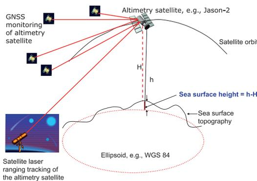
Figure 2.3: GNSS in support of monitoring changes in sea level through the determination of the altimetry satellites' precise orbit. From the precise orbital parameters, the height component  $h$  is useful in determining changes in sea level through the difference  $\{h - H\}$ , where  $H$  is measured by multiplying the speed of light with the time taken by the signals to travel from and to the satellite divided by 2, since the same distance is covered twice.
