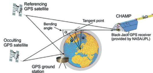
Figure 2.1: GNSS radio occultation. Use is made of (i) an occulting satellite, (ii) a non-occulting GNSS satellite and (iii) a ground-based GNSS station to determine the bending angle  $\alpha$  from which the vertical profiles of temperature and pressure are determined. Source: Wickert (2002).
