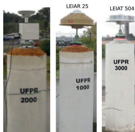
Figure 4.3: Motorized device (left) and reference antennas.
