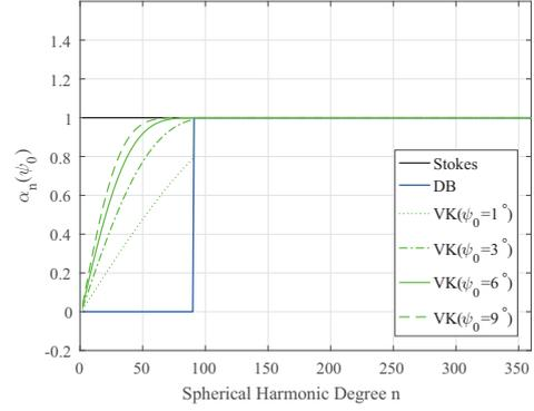
Figure 3.1: The spherical harmonic transfer coefficients of the three Stokes kernels. For the DB kernel,  $L = 90$ ;  $m_{TG} = 5400$ . For the VK kernel, the modification degree  $L = 90$  with the four different cap radii.
