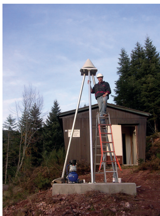
Figure 3.3: Magnetics hut and the tripod supporting the permanent, geodetic quality GPS antenna BFO1. The hut houses the DI-flux theodolite, a barometer, an infrasound sensor and a combined temperature-humidity sensor. Peter Duffner is seen during maintenance work on the GPS antenna.
