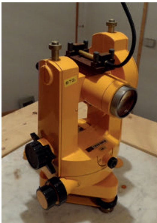
Figure 3.2: At BFO the DI-Flux theodolite is a non-magnetic Zeiss Theo-020 theodolite with a brass covered fluxgate sensing unit mounted on top of the telescope.
