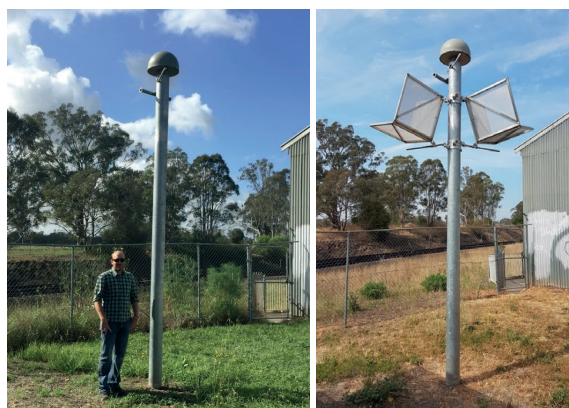
Figure 3.6: Site MENA before (left image) and after (right image) radar CRs were attached to the antenna pole
