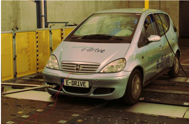
Figure 69: Vehicle being tested on the AARP
