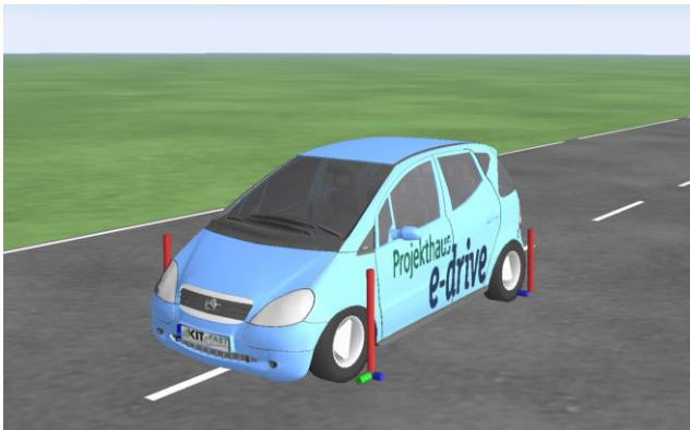
Figure 70: Vehicle in simulation software CarMaker (IPG Movie)
