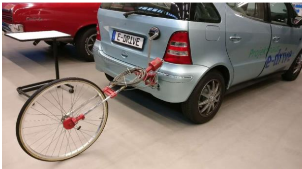
Figure 73: Peiseler wheel attached to the test vehicle
