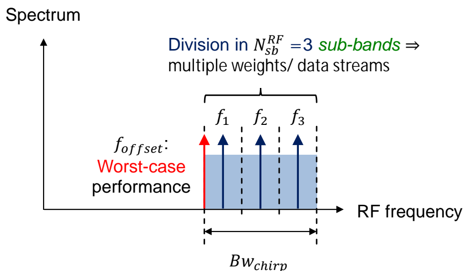
Figure 64. Schematic representation of the division of the system bandwidth into 3 sub-bands to reduce pattern mismatch at f_{offset} = f_0 - BW_{chirp}/2 = f_1 - BW_{chirp}/6 .
