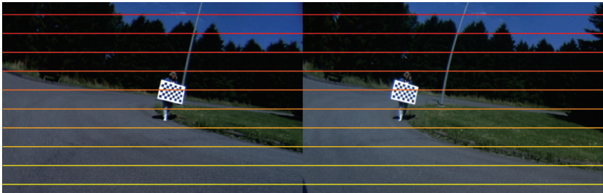
Figure 8.19: Stereo rectified image pair corresponding to Figure 8.18. For rectification the equidistant model [1] was used. One can observe that, e.g. the same tiles of the calibration target are intersected by the epipolar line. The wide baseline causes the calibration target to obstruct parts of the lamp post in the left image while being considerably offset in the right image.
