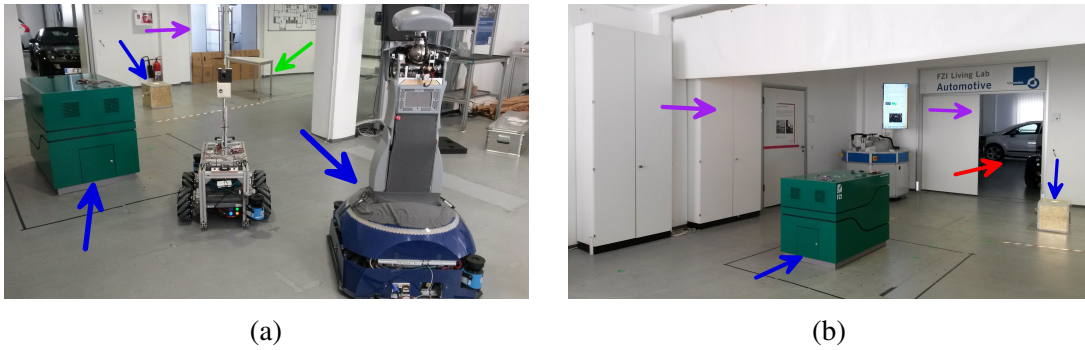
Fig. 7.8 The scenario used for the evaluation, which is captured from two angles. The blue arrows indicate the candidate objects for inspection, the green one shows the table for docking, the red one represents the doorway, and the violet ones denote the orientations of the two walls. Note that another side of the scenario is a long slope.
