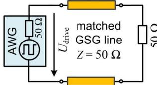
**Fig. 3.17:** Equivalent-circuit diagram of one MZM for calculation of the energy consumption. The AWG which drives the MZM is represented by an ideal voltage source and an internal resistance of  $50 \Omega$ . The GSG line of the MZM is matched to the  $50 \Omega$  output of the DAC and terminated by an external  $50 \Omega$  impedance. To estimate the energy consumption, the transmission line and its termination is replaced by an equivalent resistor of  $R = 50 \Omega$ .
