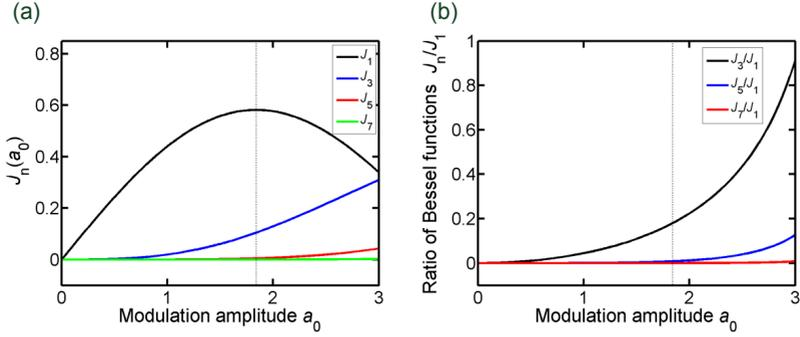
**Fig. 4.2:** (a) Plot of the Bessel functions over the modulation amplitude up to the 7<sup>th</sup> order. The modulation amplitude, where the maximum of the first order Bessel function is reached is marked with a dotted line. (b) Ratio of the different Bessel functions with respect to the first order Bessel function.
