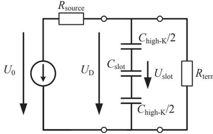
**Fig. 3.8:** Equivalent circuit of a capacitive coupled SOH phase modulator in a lumped element approximation. The source is described with the open loop voltage  $U_0$  and the source resistance  $R_{\text{source}}$ . The modulator is modeled as capacitor comprising the capacitance  $C_{\text{high-K}}$  for the dielectric and the capacitance of the slot  $C_{\text{slot}}$ . The device is terminated with  $R_{\text{term}}$ .
