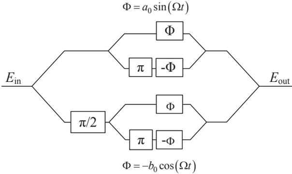
**Fig. 4.1:** Schematic of the modulator structure. To obtain a frequency shift with the SOH phase modulators, two each pair of the phase shifter is used as a Mach-Zehnder modulator (MZM) in push-pull operation. In the optical path there is a relative phase difference of  $\pi/2$  between both MZM.
