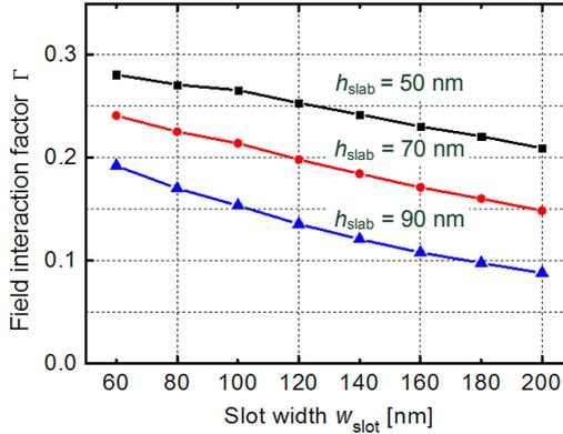
**Fig. 3.2:** Field interaction of the optical mode with the EO material in the slot  $A_{\text{slot}}$  as function of slot width at a wavelength of 1550 nm. The rail width was fixed at  $w_{\text{rail}} = 240$  nm which is approx. the optimum value for a height of the silicon layer of  $h_{\text{Si}} = 220$  nm. Thin slabs and narrow slots lead to a high field interaction factor, however, it has to be balanced with bandwidth requirements of the modulation.
