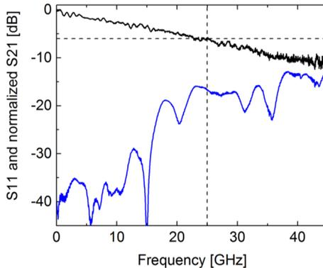
**Fig. 5.9:** EOE frequency response of a 0.4 mm long MZM. In black the normalized S21 parameter is depicted. The 6 dB point of the EOE response corresponds to the 3 dB point of the EO response and is indicated by a dashed line. The bandwidth of the device is measured to be 25 GHz. The S11 stays below 20 dB up to 20 GHz and below 15 dB up to 35 GHz, an indication for a good impedance matching to the 50 Ohm measurement system.
