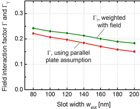
**Fig. 3.3:** Comparison between field interaction factor  $\Gamma$  and weighted field interaction factor  $\Gamma_\gamma$  for different slot widths. The slab height is  $h_{\text{slab}} = 70$  nm, the rail width  $w_{\text{rail}} = 240$  nm and the device height  $h_{\text{Si}} = 220$  nm. The weighted field interaction factor shows approximately 10% higher value than the field interaction factor calculated only with parallel plate assumption.
