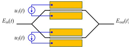
**Fig. 2.1:** Schematic of a dual drive Mach-Zehnder modulator. The incoming light is split in two arms, each of which is equipped with a phase modulator. After modulation, the light is coherently combined at the output.
