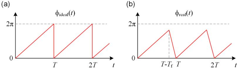
**Fig. 4.3:** (a) Illustration of an ideal sawtooth signal with period  $T$  and. The linear slope reaches from 0 to  $2\pi$ . (b) Approximation of a real sawtooth signal with fall time  $T_f$ , the slope of the signal is the same as for the ideal signal.
