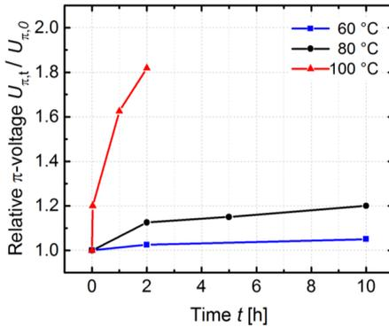
**Fig. 5.2:** Measurement of the increase in  $\pi$ -voltage over time for SOH MZM with SEO100. The devices were tested at 60 °C, 80 °C and 100 °C for 10 h. While for 100 °C a large increase is measured after the first 2 h, for 80 °C and 60 °C after a burn-in of 2 h the increase of the  $\pi$ -voltage is significantly reduced.
