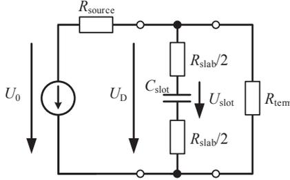
**Fig. 3.7:** Equivalent circuit of an SOH phase modulator in a lumped element approximation. The source is described with the open loop voltage  $U_0$  and the source resistance  $R_{\text{source}}$ . The modulator is modeled as RC element with the resistance  $R_{\text{slab}}$  for both silicon slabs and the capacitance of the slot  $C_{\text{slot}}$ . The device is terminated with  $R_{\text{term}}$ .
