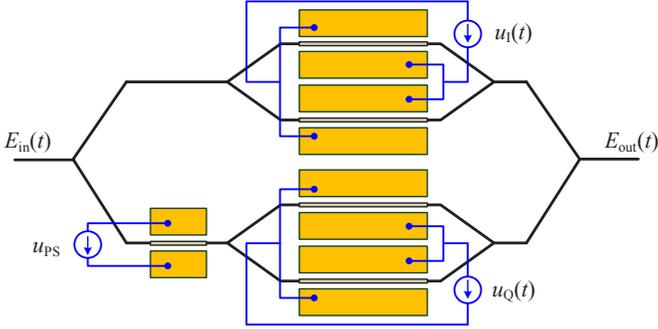
**Fig. 2.2:** Schematic of an IQ modulator. The incoming carrier is split in two arms. After inducing a relative phase shift of  $\pi/2$  using the static voltage  $u_{ps}$ , the in-phase and the quadrature component can be modulated independently by two MZM in push-pull configuration. At the output, both signals are combined. With an IQ modulator each point in the complex plane can be addressed.
