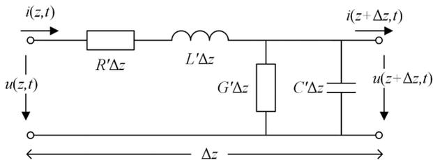
**Fig. B.1:** Equivalent circuit of a transmission line element of length  $\Delta z$ . A lumped element model is used to describe the transmission line and the evolution of the current  $i(z, t)$  and voltage  $u(z, t)$ .
