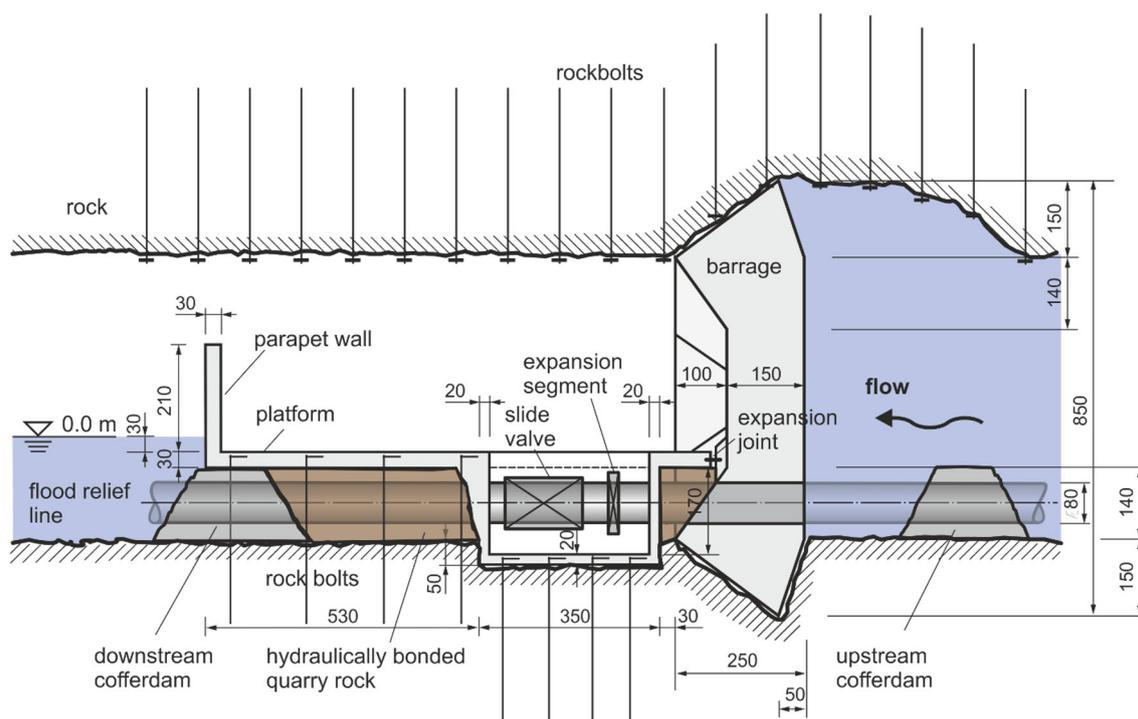
**Fig. 1** Sketch of the structure of the hydropower plant (longitudinal section, without hydraulic components) with the functional elements cofferdam, flood relief line, barrage and platform with valve chamber (Bohner et al. 2009)
