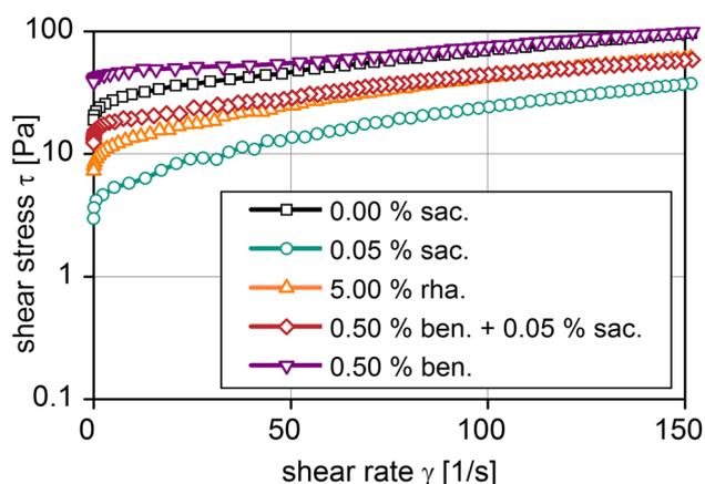
**Fig. 7** Influence of sugar (sac.), rice husk ash (rha.) and bentonite (ben.) on the flow behaviour of the cement suspensions with a water/cement ratio of 0.5 and 15 min after addition of water at atmospheric pressure and a temperature of 20 °C
