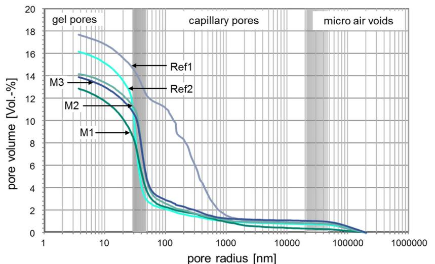
0.05 % and bentonite with 0.5 % by mass of the cement. It shows a high strength and a low porosity with only a small share of capillary pores. By increasing the sand content, the higher cement content due to the lower water/cement-ratio was compensated. Compared to the Indonesian reference mixture, even a reduction of the cement content of 10 % was achieved while maintaining the known workability.
