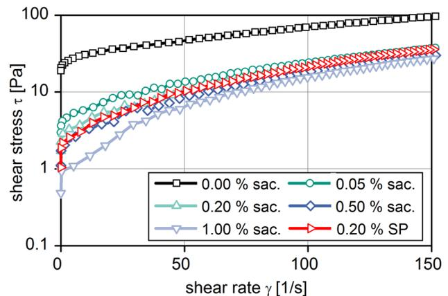
**Fig. 6** Influence of sugar (sac.) and superplasticizer (SP) on the flow behaviour of the cement suspensions with a water/cement ratio of 0.5 and 15 min after addition of water at atmospheric pressure and a temperature of 20 °C
