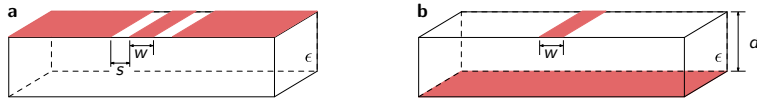
Figure 3.2: Planar implementations of transmission lines (a) Coplanar line with central conductor of width w and ground reference in the device plane at a spacing s . The substrate has a dielectric constant \epsilon \sim 11 for intrinsic silicon and sapphire, which are substrate materials commonly used for fabricating superconducting quantum circuits. (b) Microstrip line with single conductor of width w and a ground plane on the backside of the substrate. The thickness d of the substrate gives the distance to the ground reference.
