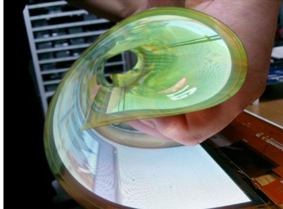
**Figure 1.0.1:** A flexible OLED Display manufactured by the Korean manufacturer LG (source: [www.digitaltrends.com](http://www.digitaltrends.com))
