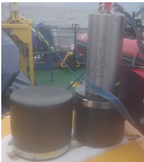
Figure 2.6.: Photograph of Evologics S2C 7/17 USBL modems by Evologics. Made during trials in the baltic sea. The left modem is the one mounted to the AUV, the right one was temporarily attached next to it for quick in-air testing (this should be done with care as it may harm the transmitters).
