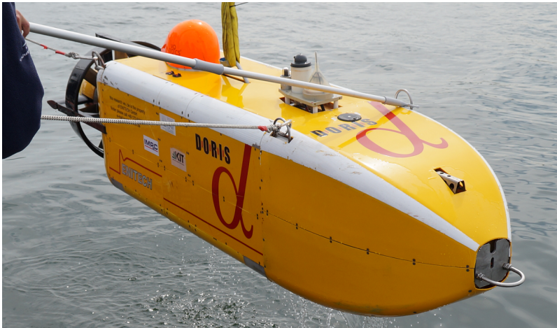
Figure 2.1.: Photograph of the SMIS AUV being recovered from the water during tests at Lake Constance in May 2016. The orange bulb in the back covers the USBL modem for mechanical protection and hydrodynamics (Picture courtesy of IMPaC GmbH, Hamburg).
