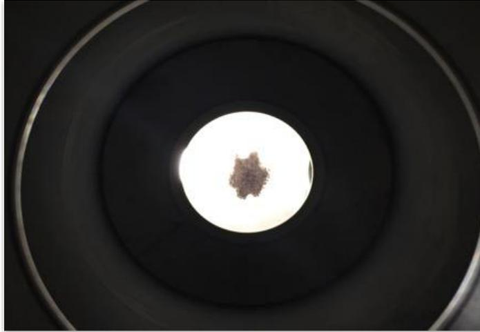
**Fig. 1.2.18:** Thermal paper shot at the back side of the microwave load (at the position where the conical mirror is mounted).
