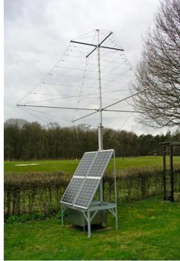
**Figure 3.29:** A radio station prototype. The log-periodic dipole antenna and solar panels are visible. The electronics and digitizer are placed in the aluminum box beneath it [225].
