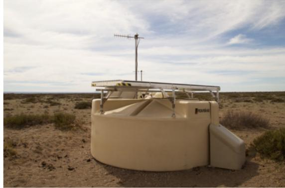
**Figure 3.31:** One SSD module already installed in the Pierre Auger Observatory [228].
