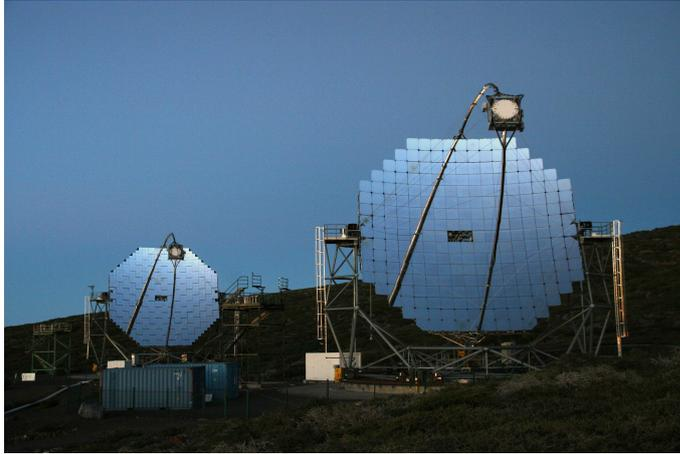
**Figure 1.17:** The two 17 m diameter MAGIC telescope system operating at the “Roque de los Muchachos” observatory in La Palma. The front telescope is the MAGIC-II [92].
