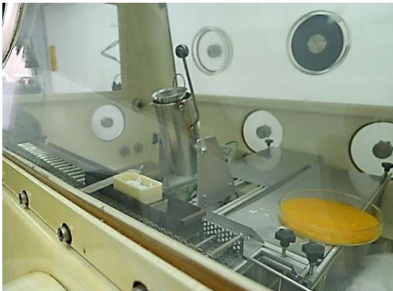
**Fig. 2.8.1:** Na heating and filling pot located in glovebox.
