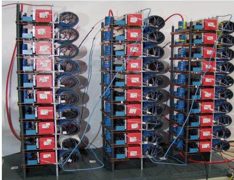
**Fig. 2.7.3:** Pulse generator comprising 30 modules.
